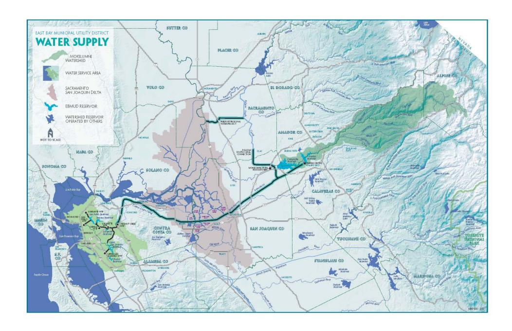
Streamflow from the Mokelumne River is collected and stored in the District's Pardee and Camanche Reservoirs, located in the Sierra foothills. Raw water from Pardee Reservoir is transported to the East Bay terminal reservoirs and treatment plants through the Pardee Tunnel, the three Mokelumne Aqueducts, and the Lafayette Aqueducts. The raw water is treated at one of the District's treatment plants before being delivered to customers.
