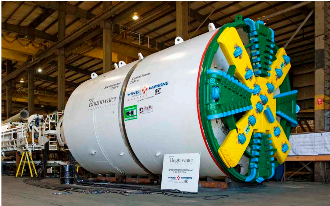
Figure A5. Slurry TBM Fitted with Disc Cutters (Brightwater BT-3)
