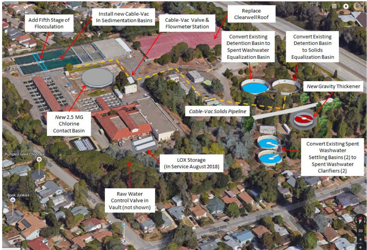
Figure 2 – Aerial View of USL WTP Proposed Improvements
