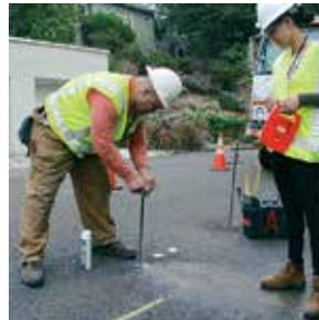
Another tool used in the field is an audiometric correlator, which helps crews locate the position of a leak. The correlator works in tandem with microphones that are placed at two test points a known distance apart along a water pipe. By measuring changes in sound that the leak
