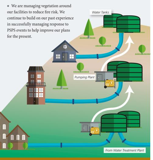
EBMUD has more than 122 pressure zones, which require power to pump water to higher elevations. During PSPS, tanks are filled with water at or near capacity
