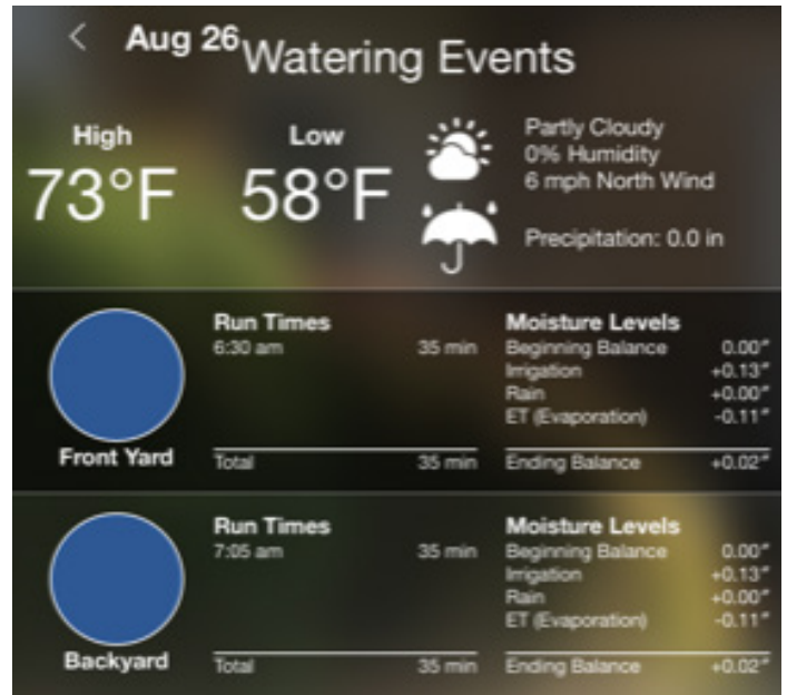
Irrigation adjusted based on weather
