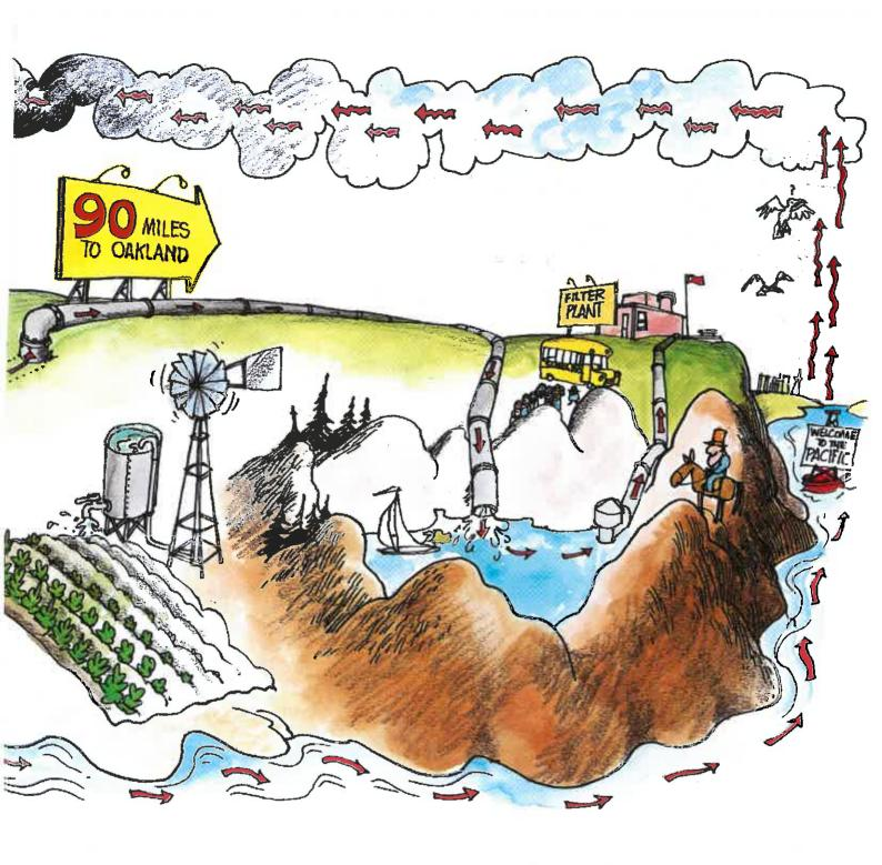
Water from Pardee Reservoir travels to the East Bay cities through three big pipes (called the Mokelumne Aqueducts). The pipes go 90 miles across California. The biggest pipe is seven feet across—big enough for a grown-up to walk in. The water flows through the pipes without being pushed through. It takes two days for the water to go from Pardee Reservoir to the East Bay. Sometimes big pumps push the water through the pipes faster when more water is needed in the East Bay.
