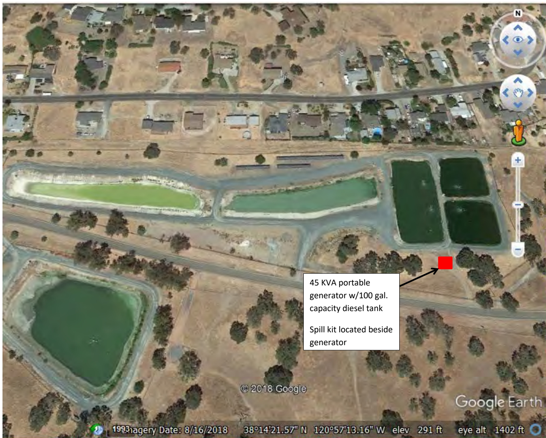
Camanche North Shore Wastewater Treatment Plant Map depicting location of portable generator leased for potential PG&E PSPS Events
