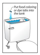
the toilet tank. A flapper test will tell you if the flapper valve is leaking. To complete a flapper test, you will need some food coloring or dye tabs. Put enough food coloring into the toilet tank to change the color (5 drops or 2 dye tabs) and then replace the tank lid. Wait 20 minutes. See how to video
