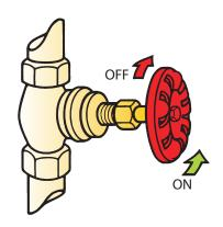
**Step 2** After you have turned off the house line shut-off valve, line up a toothpick or a pin with the hand of the meter, as before. Wait 30 minutes, and then look at the water meter dial.
