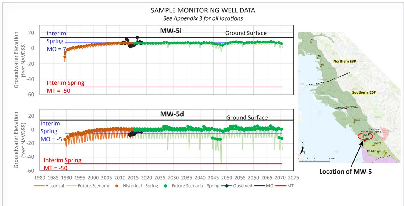
These hydrographs depict observed and modeled intermediate and deep aquifer zone groundwater elevations at MW-5 over time with associated land subsidence minimum thresholds and measurable objectives, based on using groundwater levels as a proxy for land subsidence. Similar land subsidence hydrographs with sustainable management criteria for other RMS wells are presented in Appendix 3.D.
