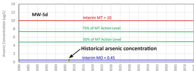
These time-series plots of chloride (secondary MCL) and arsenic (primary MCL) show historical baseline concentrations with associated minimum thresholds and measurable objectives. In addition, key constituents with primary MCLs such as arsenic have been assigned Action Levels set at 50% and 75% of the MT. Time-series plots for other RMS wells are provided in Appendix 3.E.
