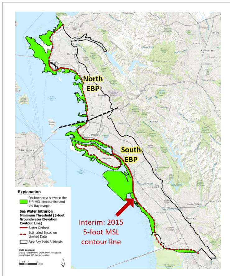
The seawater intrusion sustainable management criteria are based in part on monitoring potential inland movement of the shallow aquifer five feet groundwater elevation contour (i.e., inland expansion of green area on this figure, which represents the area between San Francisco Bay margin and the five-foot groundwater elevation contour).
