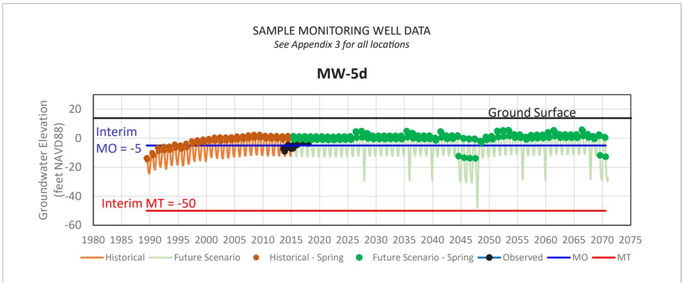
This hydrograph depicts observed and modeled deep aquifer zone groundwater elevations at MW-5 over time with associated groundwater level minimum thresholds and measurable objectives. Similar groundwater level hydrographs with sustainable management criteria for other RMS wells are presented in Appendix 3.A.
