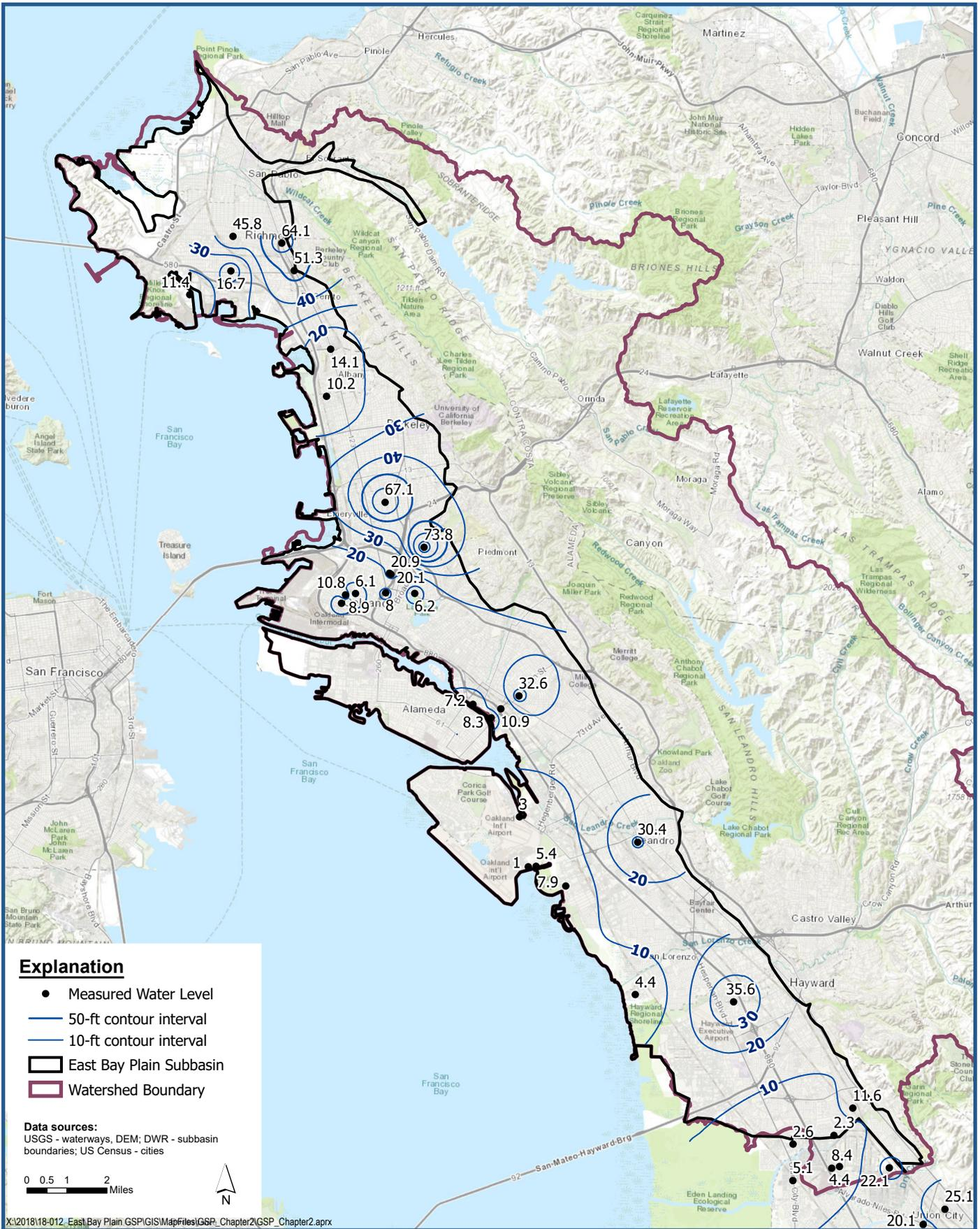
**Water Table Aquifer Groundwater Elevation
