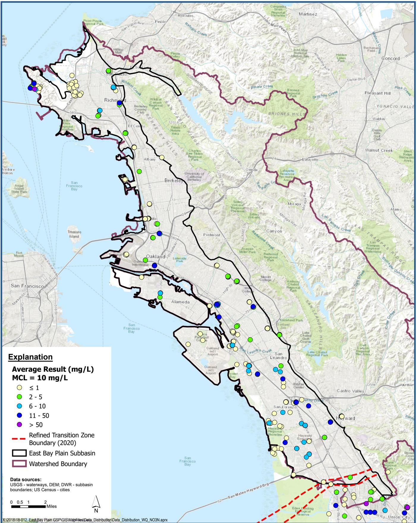
**Average Nitrate (NO<sub>3</sub>N) Measurement for Wells Deeper than 50-feet**
