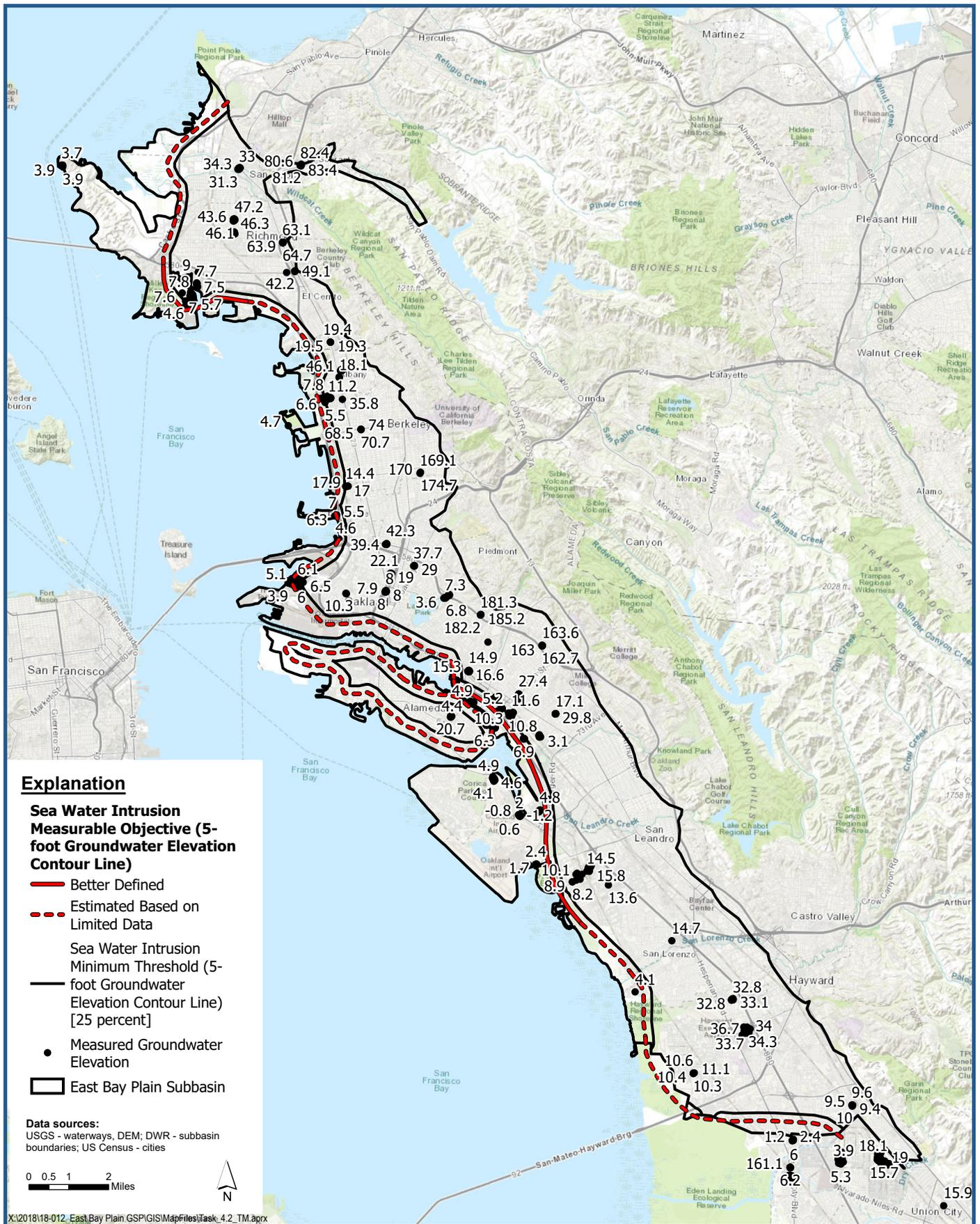
**Seawater Intrusion Minimum Threshold and Measurable Objective**
