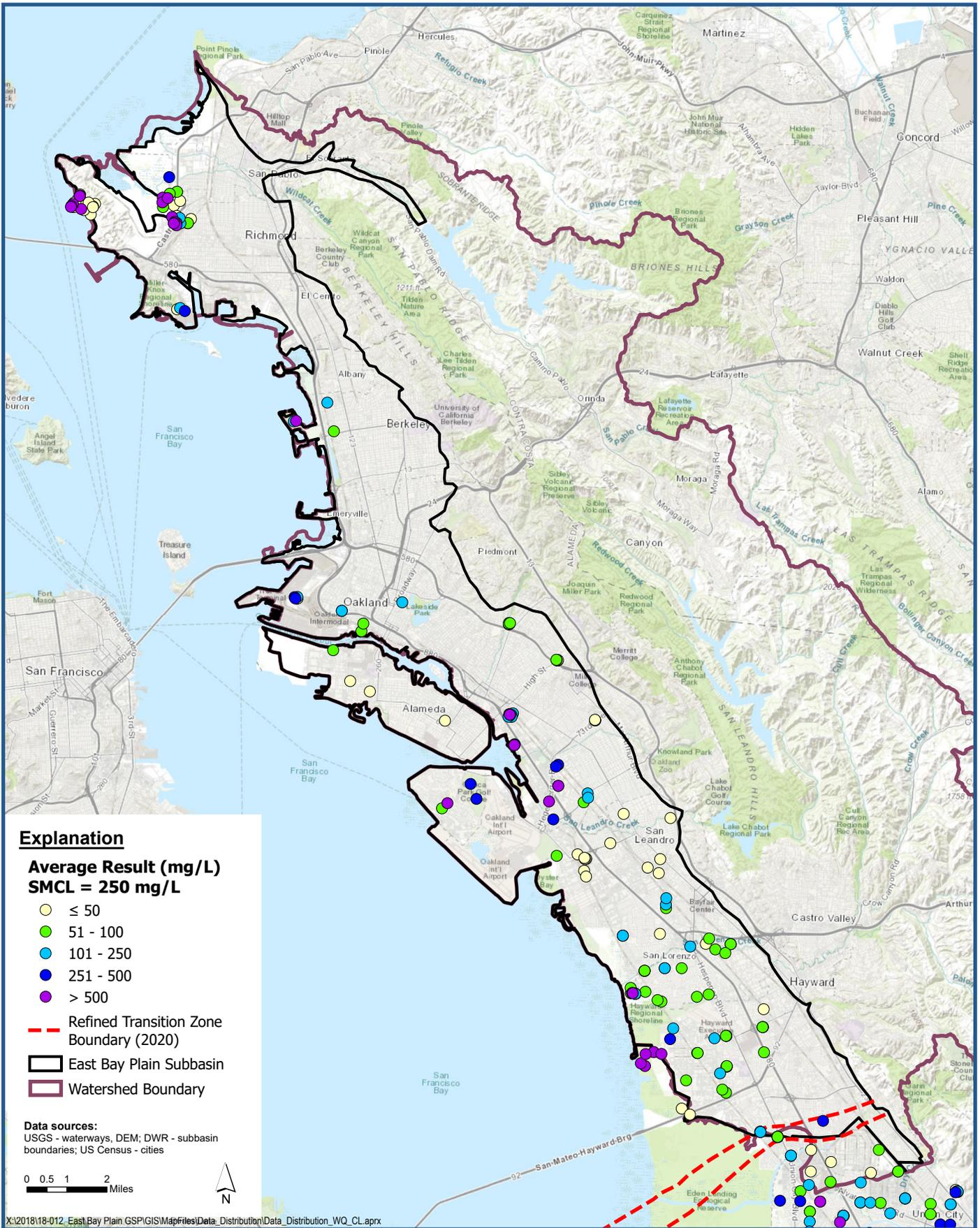
**Average Chloride (Cl) Measurement for Wells Deeper than 50-feet**
