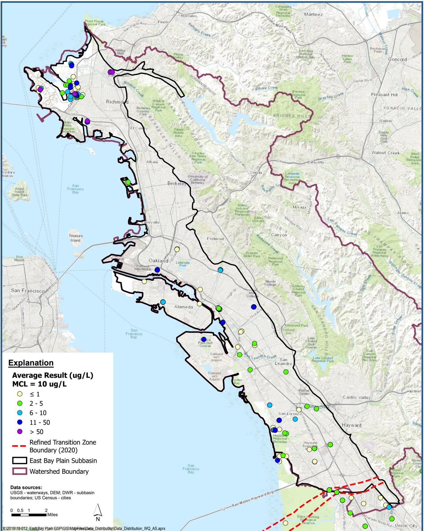
**Average Arsenic (As) Measurement for Wells Deeper than 50-feet**
