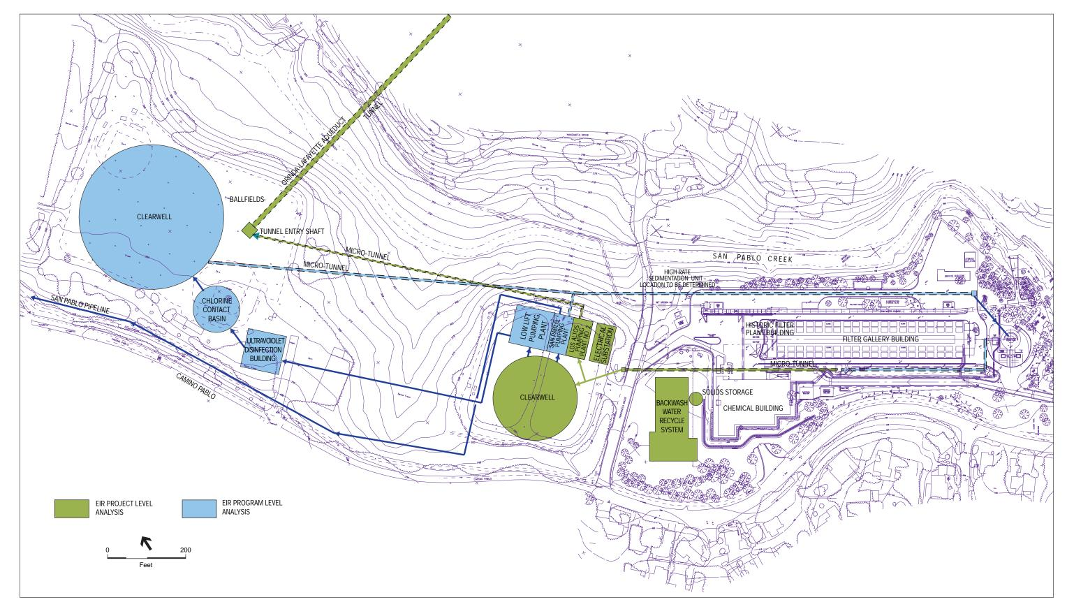
EBMUD Water Treatment and Transmission Improvements Program . 204369 Figure 6-2 Modified Orinda WTP Site Plan Alternative
