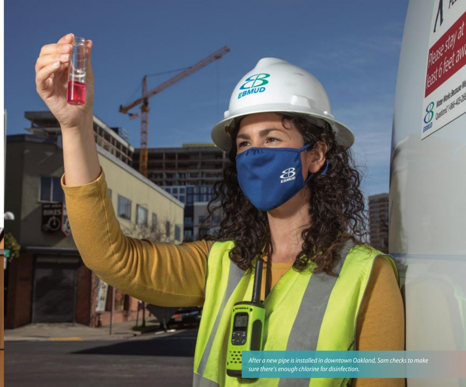
After a new pipe is installed in downtown Oakland, Sam checks to make sure there's enough chlorine for disinfection.
