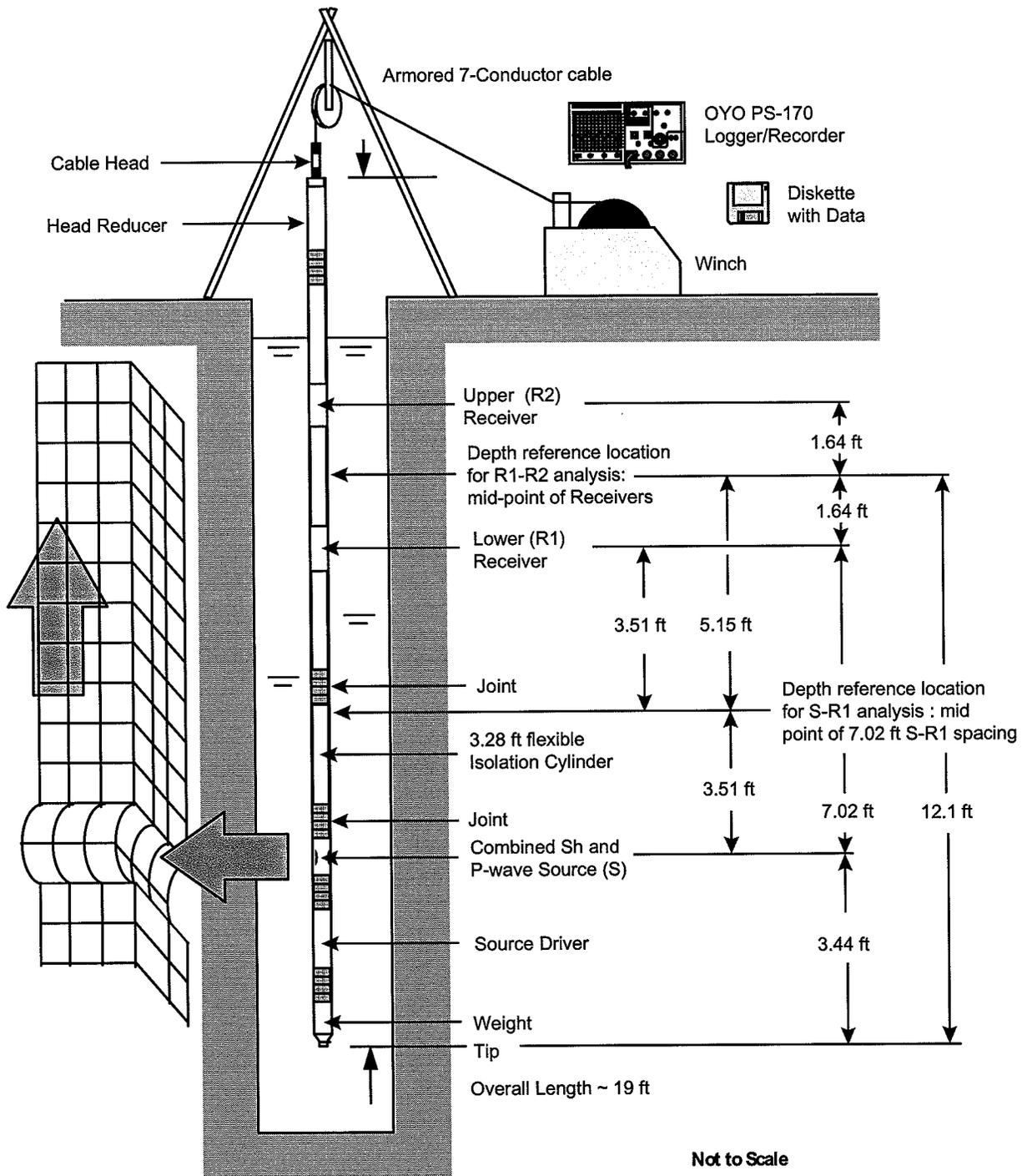
Figure 1. Concept illustration of P-S logging system
