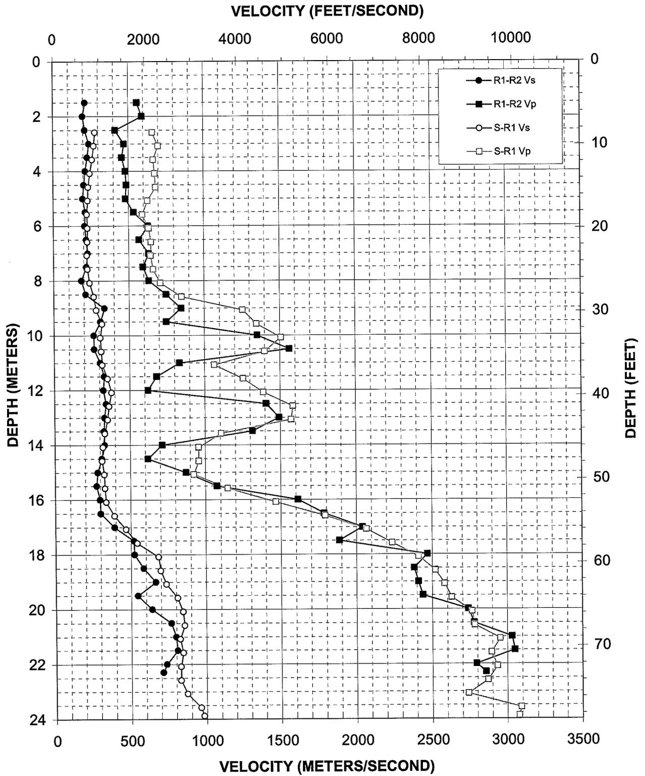
Figure A-1. Boring VQ-38, R1 - R2 high resolution analysis and S-R1 quality assurance analysis P- and S<sub>H</sub>-wave data
