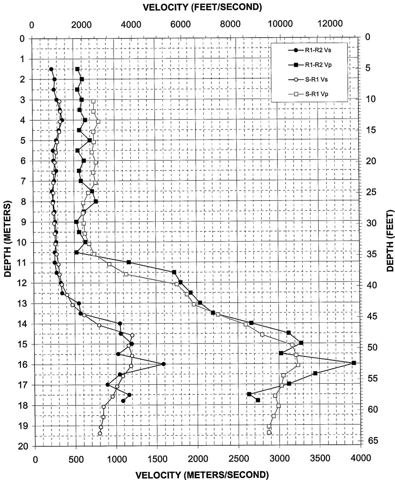
Figure A-2. Boring VQ-40, R1 - R2 high resolution analysis and S-R1 quality assurance analysis
