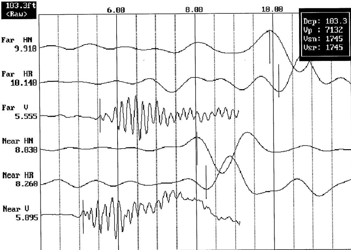
Figure 2. Example of filtered (1400 Hz lowpass) record
