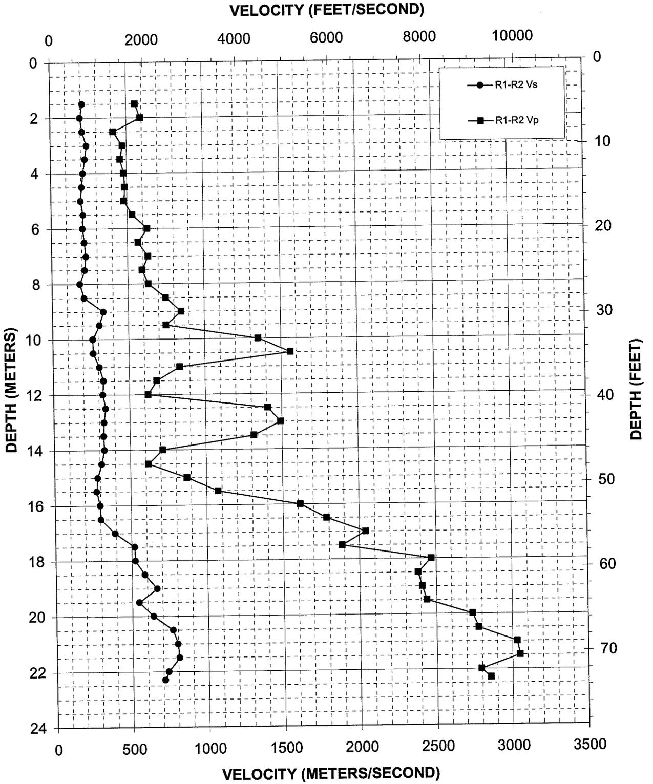
Figure 4. Boring VQ-38, Suspension P- and S<sub>H</sub>-wave velocities
