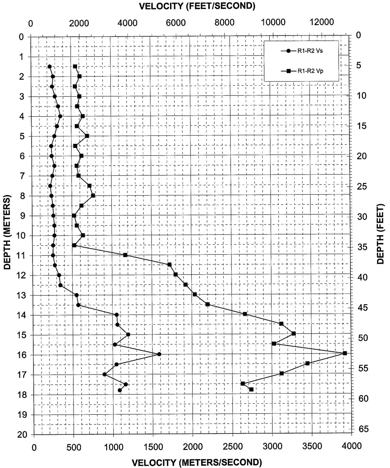
Figure 5. Boring VQ-40, Suspension P- and S<sub>H</sub>-wave velocities
