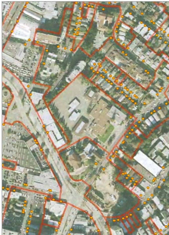
The base year polygon demands were calculated using the Demand Model. The process of spatially calculating demands is presented on Figure 4.5, Calculation and Distribution of Base Year Demands. Each of the approximately 22,000 land use polygons (8,300 before overlying the polygons with DMR, slope, and pressure zone boundaries) has a demand associated with it.
