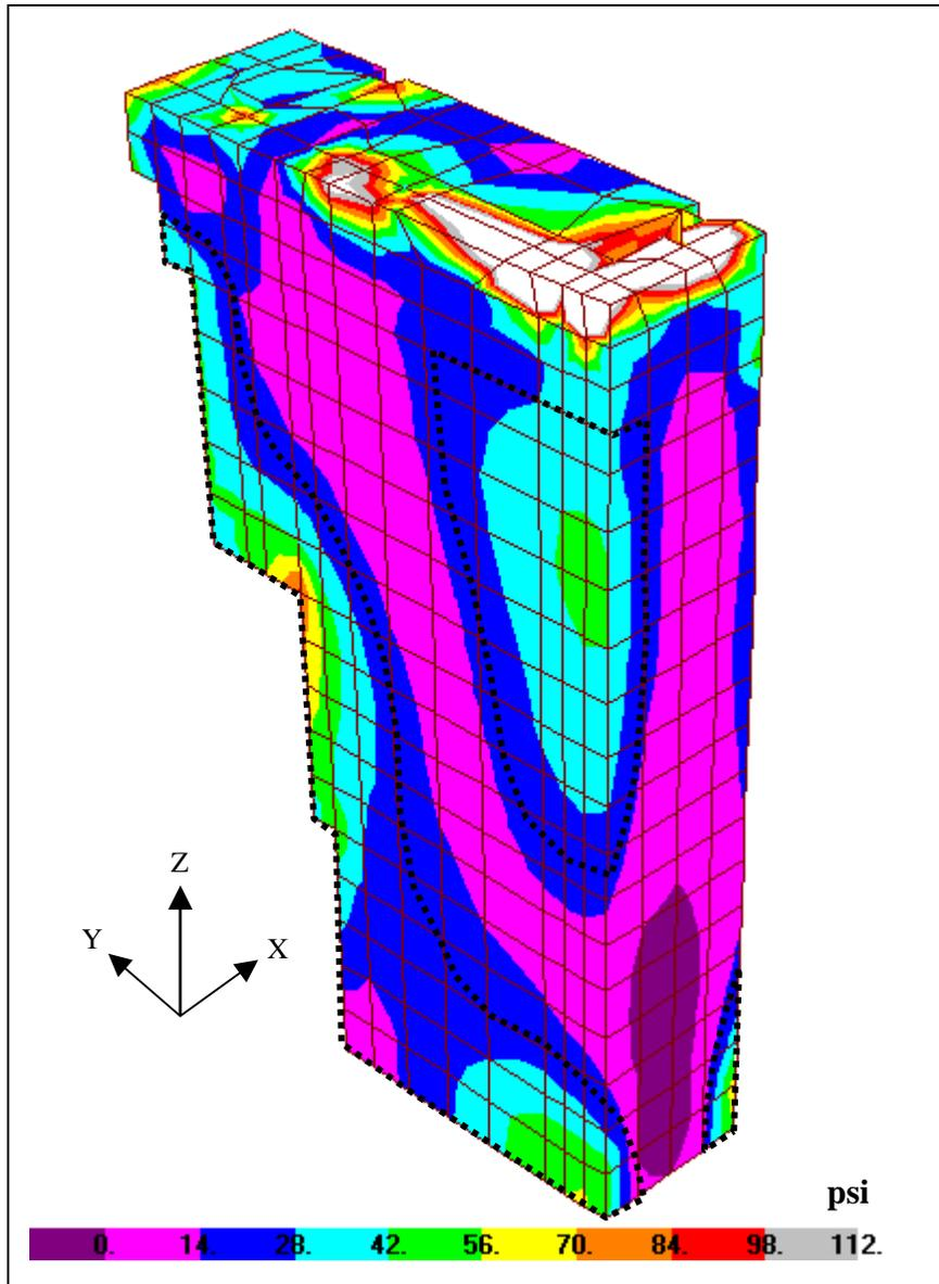
**Figure 5-13a:** Maximum vertical stresses ( $\sigma_{zz}$ ) in the south wall due to static plus earthquake loads. Regions within the dotted lines indicate potential tension failure.
