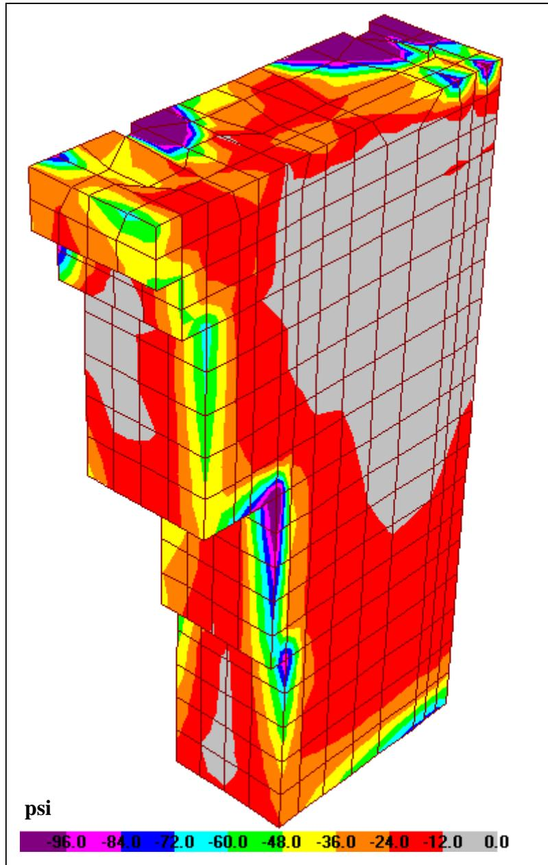
**Figure 5-11b:** Minimum horizontal normal stresses ( $\sigma_{xx}$ ) for the south wall due to static minus earthquake loads.
