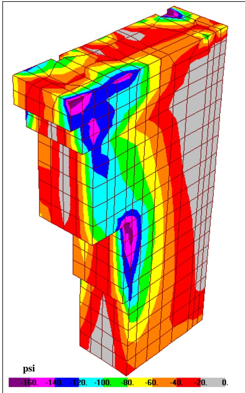
**Figure 5-12b:** Minimum horizontal normal stresses ( $\sigma_{yy}$ ) in the south wall due to static minus earthquake loads.
