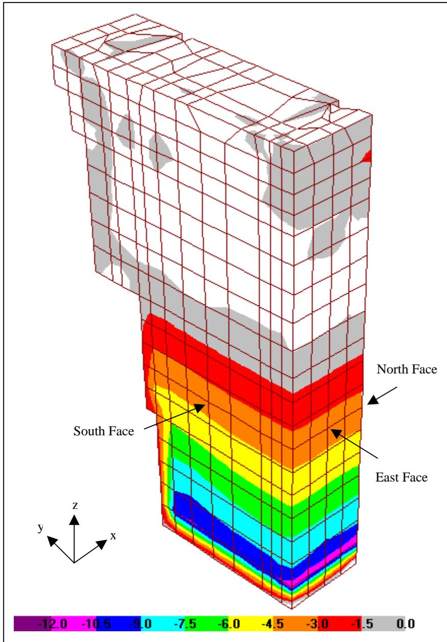
**Figure 5-9a:** South-wall horizontal stresses ( $\sigma_{xx}$ ) due to hydrostatic pressures (psi)
