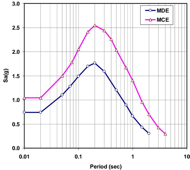
**Figure 3-2:** Comparison of MCE with MDE Horizontal Spectral Accelerations at 5% damping
