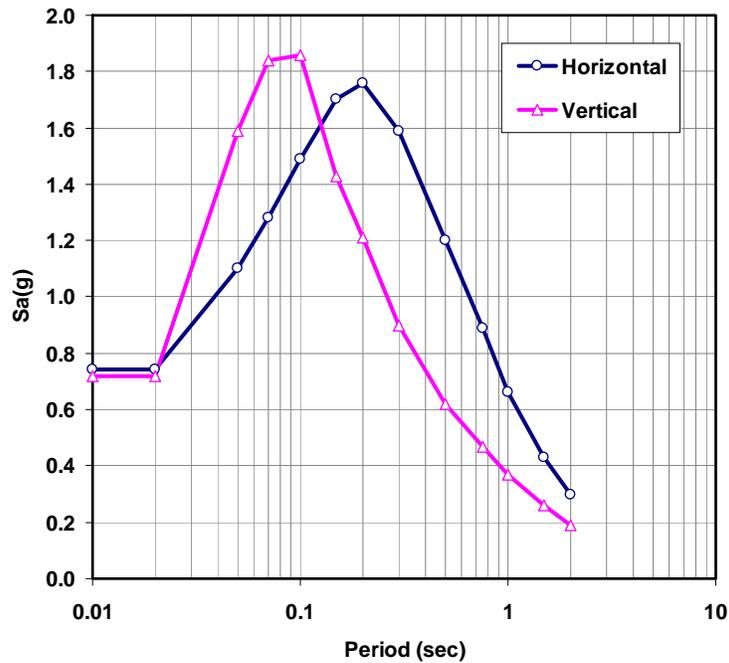
**Figure 3-1: MDE Horizontal and Vertical Spectral Accelerations at 5% damping**
