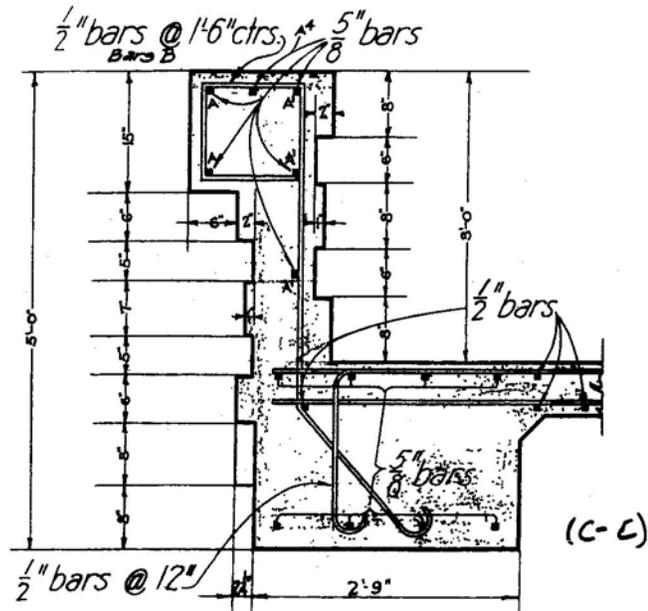
**Cross-Section of Pavilion Roof Beam**
