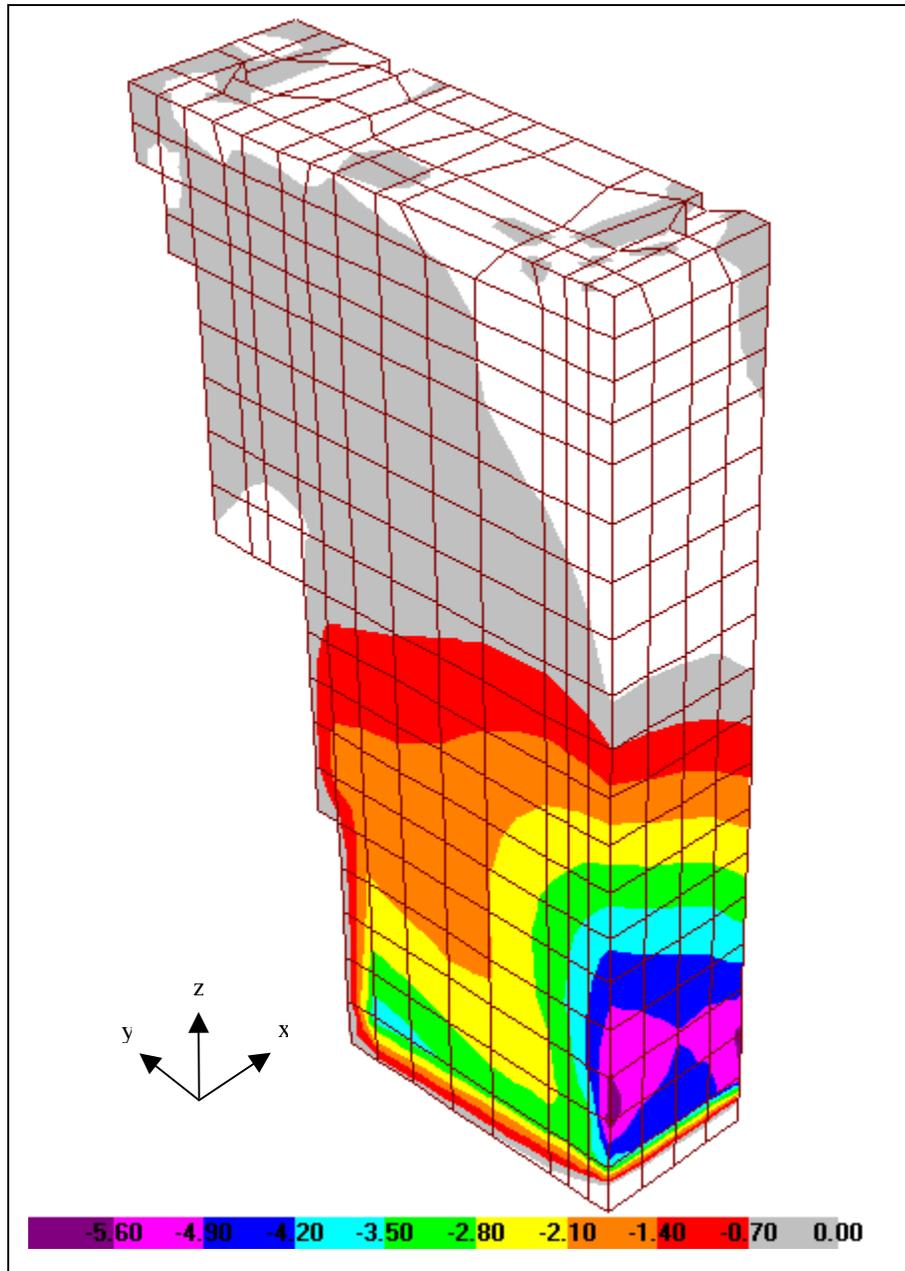
**Figure 5-9c:** South-wall vertical stresses ( $\sigma_{zz}$ ) due to hydrostatic pressures (psi)
