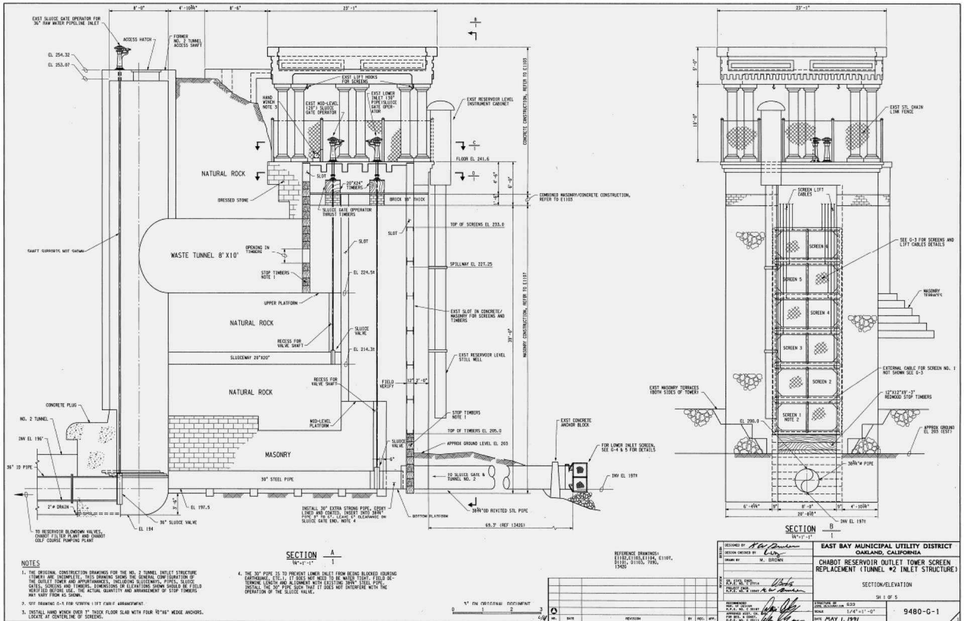
**Figure 2-2:** Section/elevation view showing multi-level entry portal structure and 8-foot brick-lined outlet shaft
