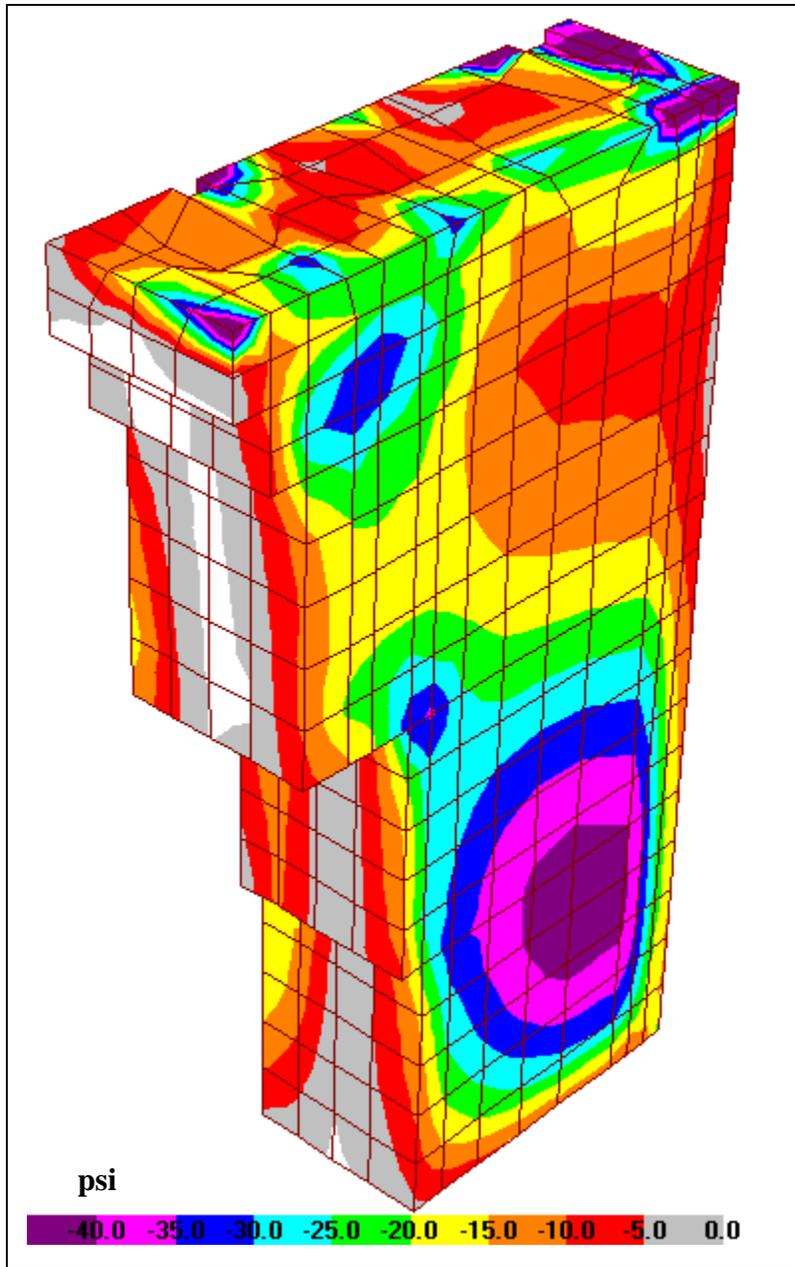
**Figure 5-15b:** Minimum in-plane shear stresses ( $\sigma_{yz}$ ) in the south wall due to static minus earthquake loads
