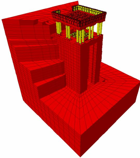
**Figure 5-1:** Front view of the tower, foundation, abutment, and pavilion model
