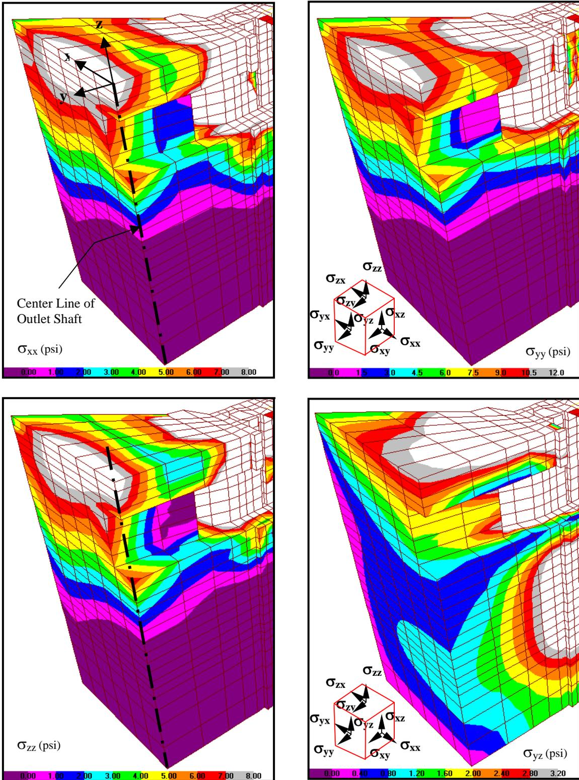
**Figure 5-17:** Normal and shear stresses in the vicinity of the outlet shaft
