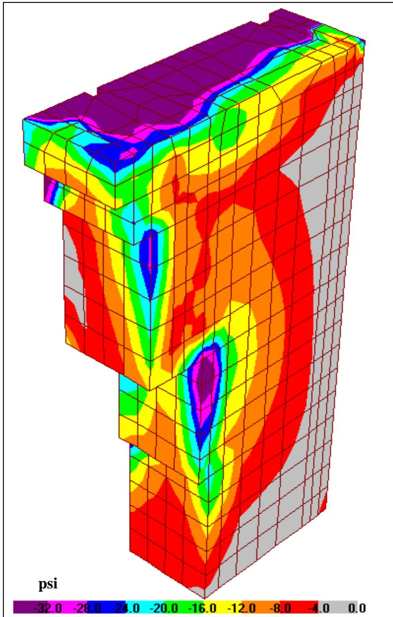
**Figure 5-14c:** Minimum out-of-plane shear stresses ( $\sigma_{xy}$ ) for the south wall due to static minus earthquake loads
