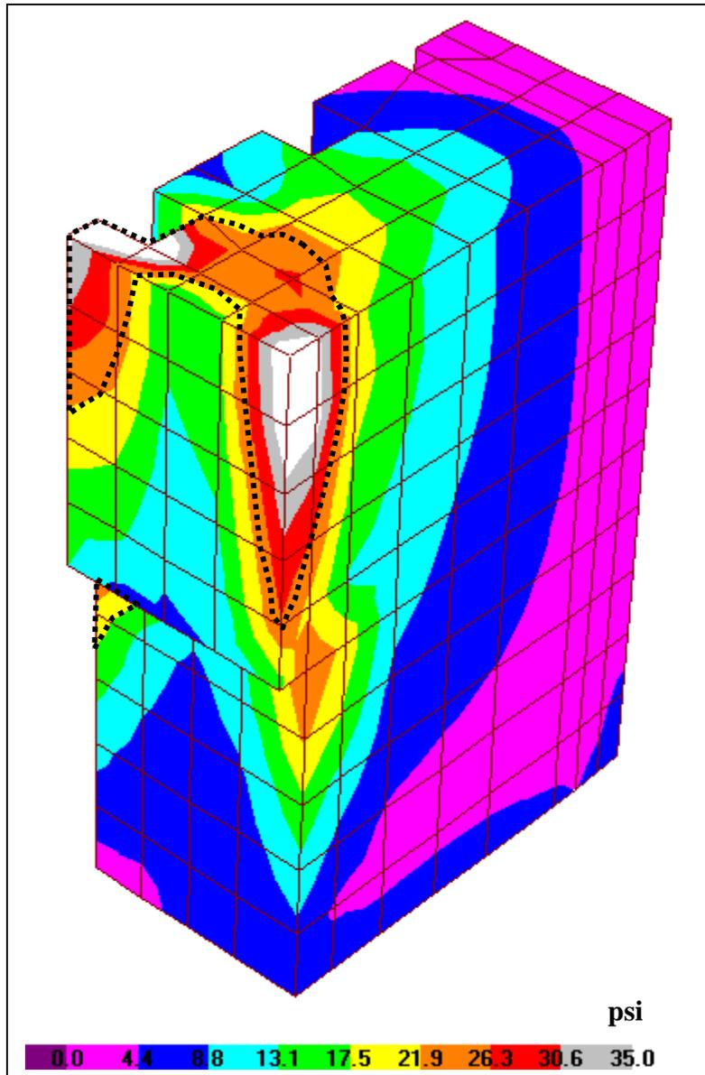
**Figure 5-14b:** Maximum out-of-plane shear stresses ( $\sigma_{xy}$ ) on bottom half of the south wall due to static plus earthquake loads.
