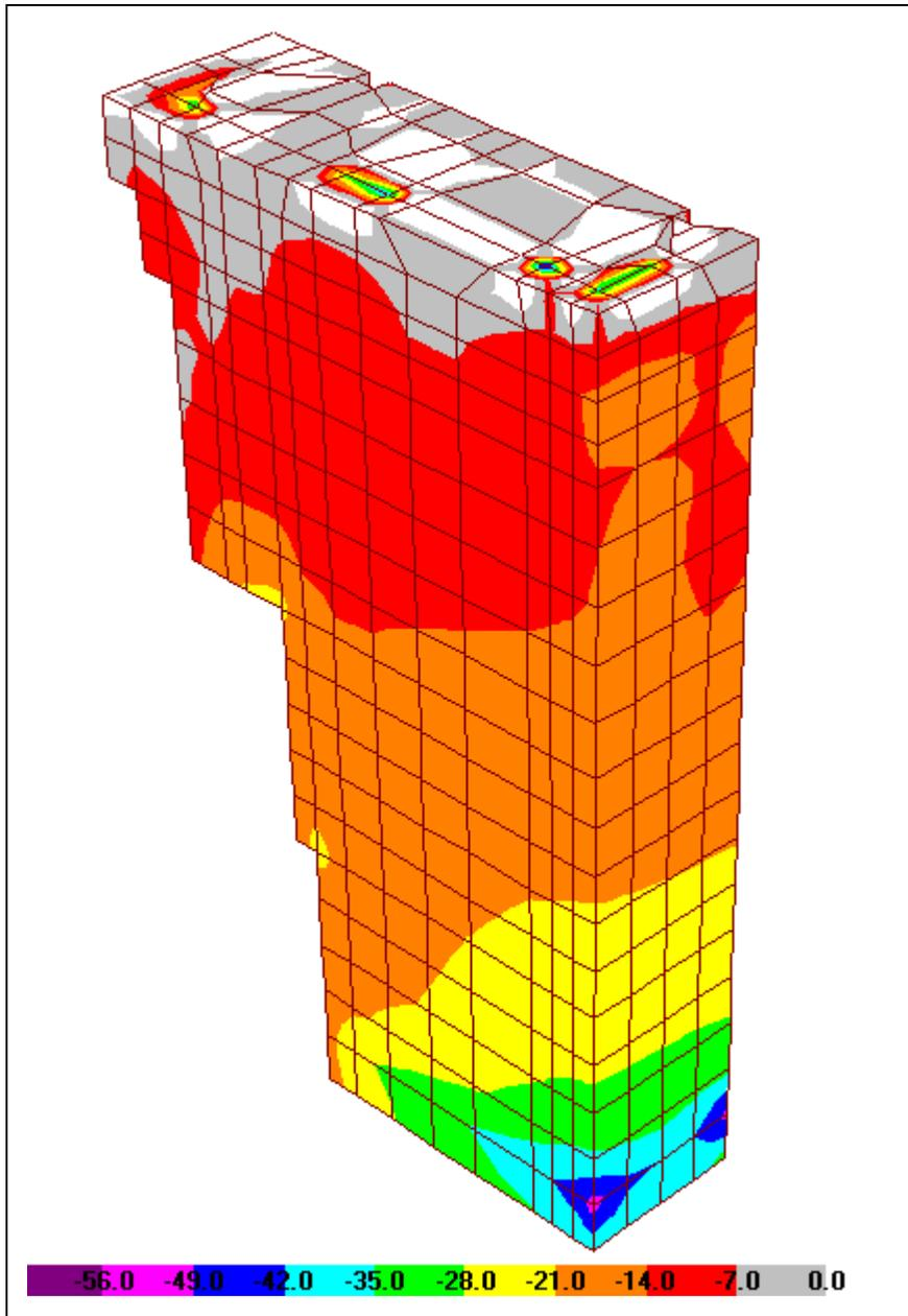
**Figure 5-8:** South-wall vertical stresses due to self weight (psi)
