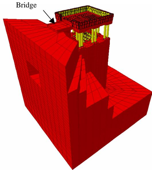
**Figure 5-2:** Back view of the tower, foundation, abutment, and pavilion model
