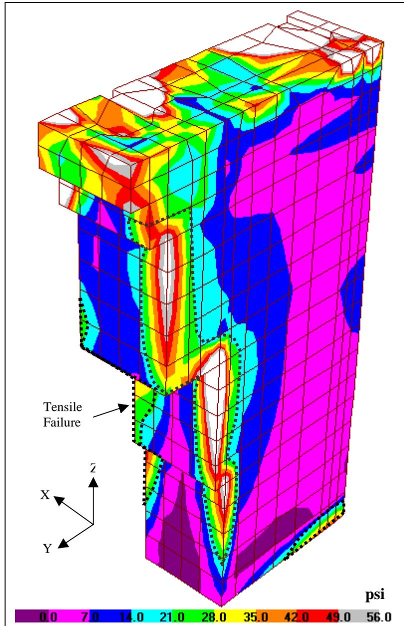
**Figure 5-11a:** Maximum horizontal normal stresses ( $\sigma_{xx}$ ) for the south wall due to static plus earthquake loads. Regions within the dotted lines indicate potential tension failure.
