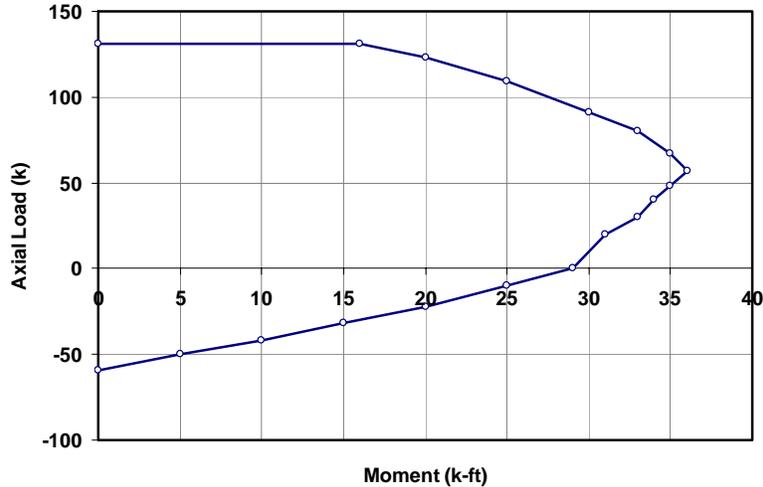
**Figure 4-1:** Axial load-bending moment interaction diagram for pavilion columns
