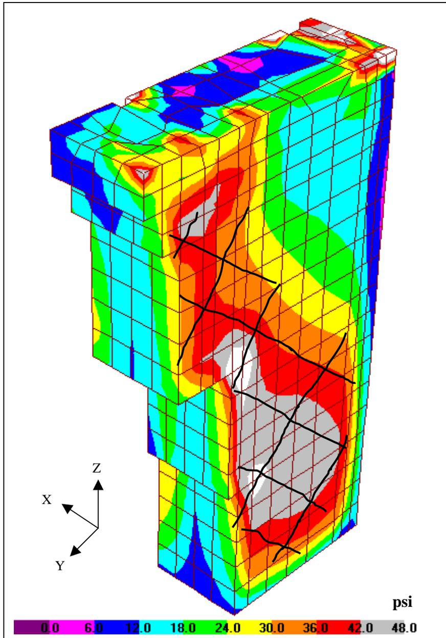
**Figure 5-15a:** Maximum in-plane shear stresses ( $\sigma_{yz}$ ) in the south wall due to static plus earthquake loads
