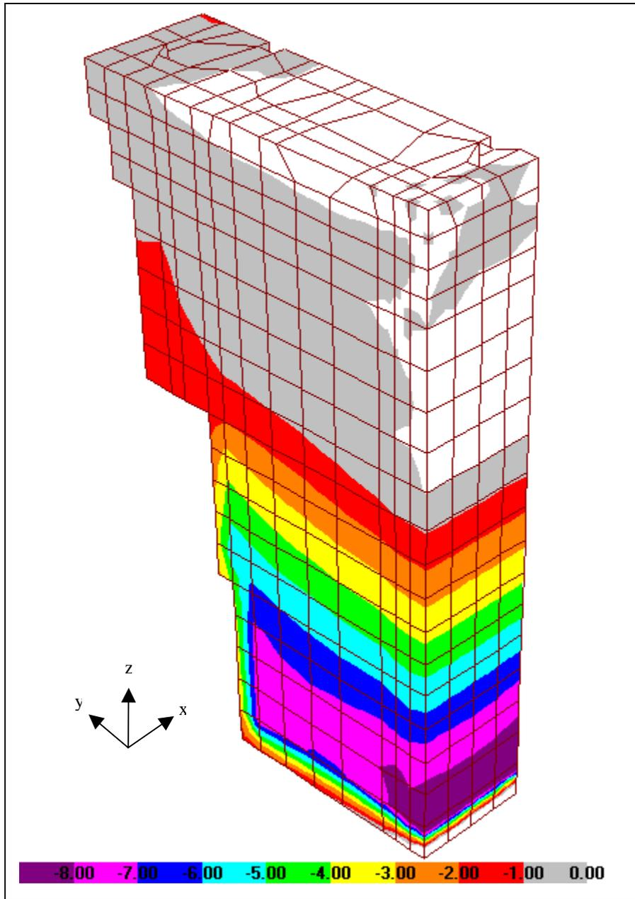
**Figure 5-9b:** South-wall horizontal stresses ( $\sigma_{yy}$ ) due to hydrostatic pressures (psi)
