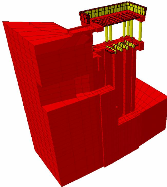
**Figure 5-7:** Vertical mid-section view showing stop timber slots and 8' x 10' waste tunnel. Also shown are pavilion roof beams and slab and floor beams and slab.
