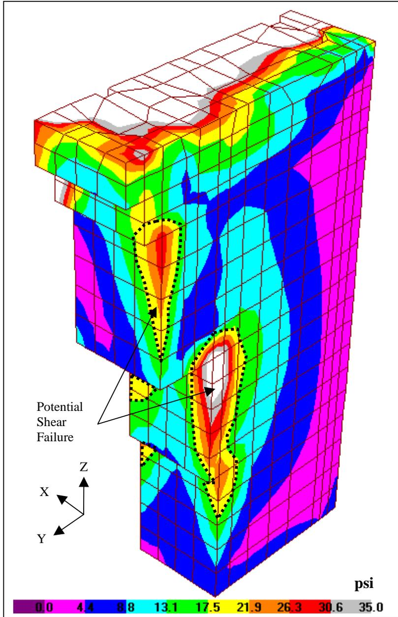
**Figure 5-14a:** Maximum out-of-plane shear stresses ( $\sigma_{xy}$ ) for the south wall due to static plus earthquake loads.
