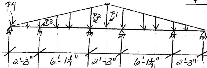
$$\text{Parapet} \rightarrow W_{DL} = 0.15 \text{ k/ft}^3 (1.5 \text{ ft}) (1.25 \text{ ft}) + 0.15 \text{ k/ft}^3 (1 \text{ ft}) (3 \text{ ft} - 1.25 \text{ ft})$$
