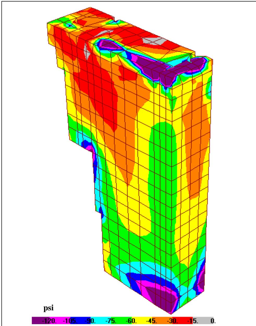
**Figure 5-13b:** Minimum vertical stresses ( $\sigma_{zz}$ ) in the south wall due to static minus earthquake loads.
