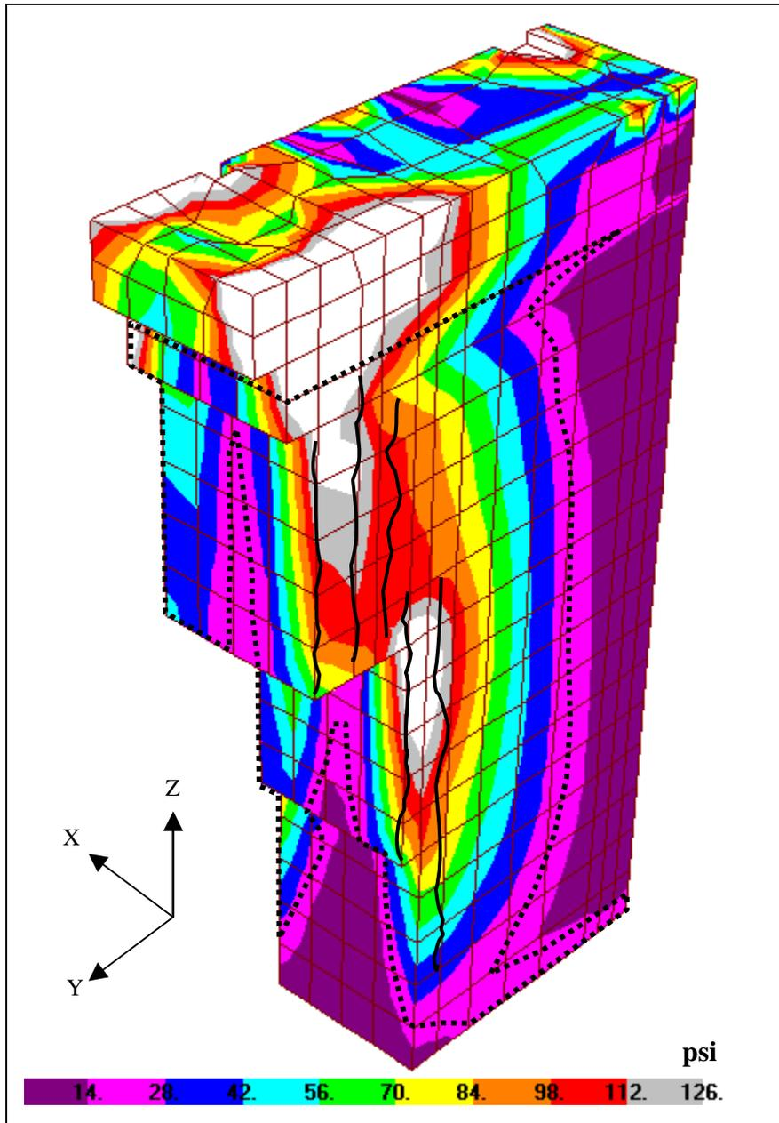
**Figure 5-12a:** Maximum horizontal normal stresses ( $\sigma_{yy}$ ) for the south wall due to static plus earthquake loads. Regions within the dotted lines indicate potential tension failure.
