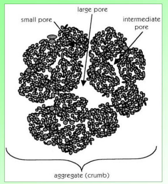
A well aggregated soil has a range of pore sizes. This medium size soil crumb is made up of many smaller ones. Very large pores occur between the medium size aggregates. <u>Occurs</u> physically and biologically.
