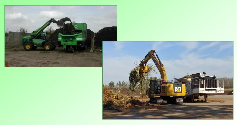
Feedstock preparation: grinding (and mixing if food waste, etc.)
