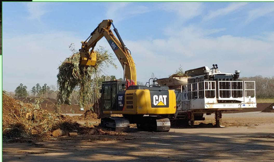
Feedstock preparation: grinding (and mixing if food waste, etc.)
