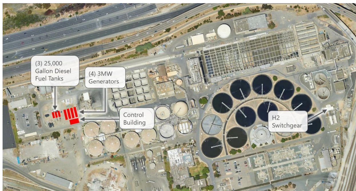
FIGURE 3-4: PROJECT 4 - 12 MW GENERATOR
