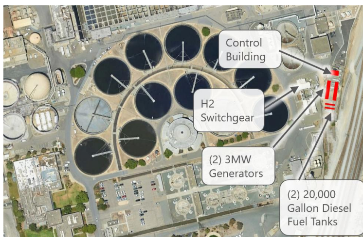
FIGURE 3-5: PROJECT 5 - 6 MW GENERATORS
