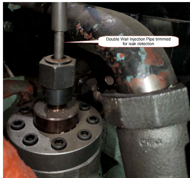
Figure 36: Modified High Pressure Fuel Injection Line
