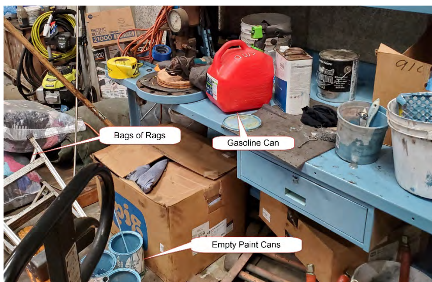
Figure 31 - Gasoline Stored Adjacent to Combustibles
