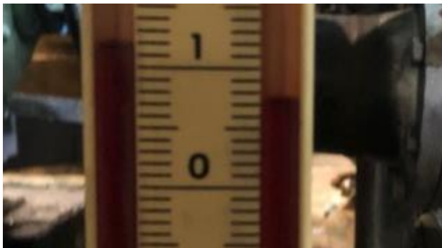
Crankcase vacuum at 2300 kw dual fuel.
