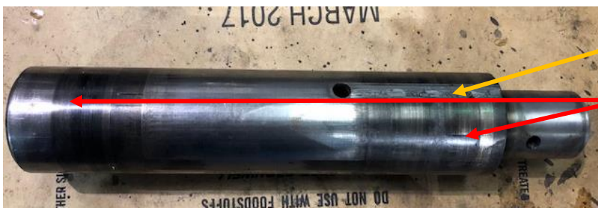
Scratch from disassembly
