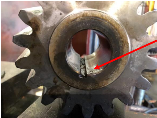
Rear side of gear blue steel and heat pitting (seized area).
