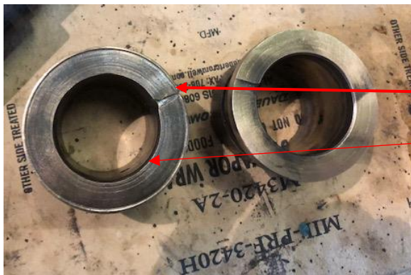
Both bushings have fine cuts from debris. (Should be smooth from years of lubricated operation)
