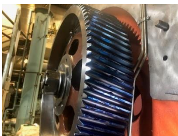
Camshaft to idler gear teeth blue pattern
