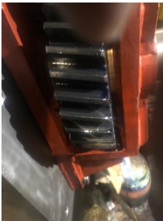
Oil pump gear teeth blue pattern
