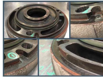
Fig. 4: Damaged axial and circumferential cam recess.
