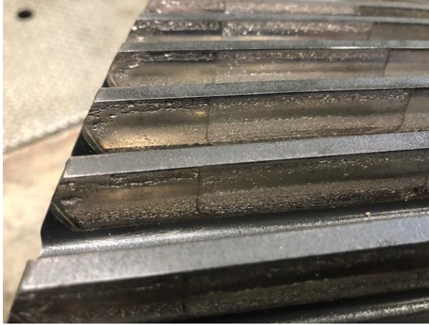
Water Pump Drive Gear Damage
