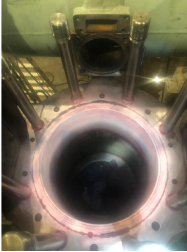
#3 cylinder upper bore die penetrant inspection with piston still in bore. (no sign of crack or leaks)
