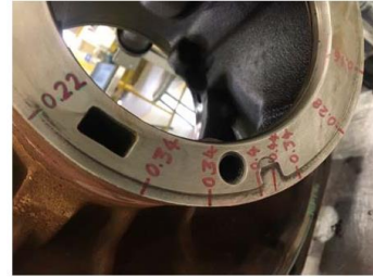
Fig. 2: Worn out sealing cover clamping area.
