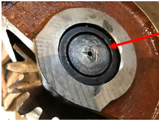
Bushing and shaft seized together with coked oil between the shaft and bushing.
