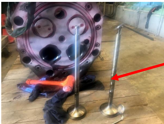
Oily water on valve stem
