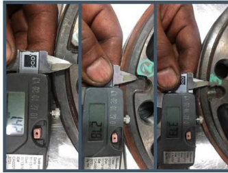
Fig. 1: Worn out cam recess.
