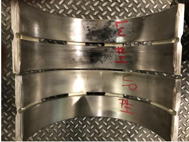
#5 Main bearing loading and overlay fatigue on lower shell
