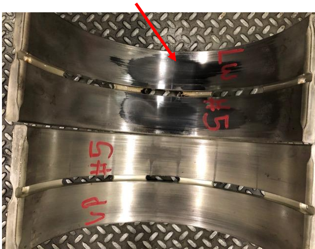
#5 Main bearing loading and overlay fatigue on lower shell
