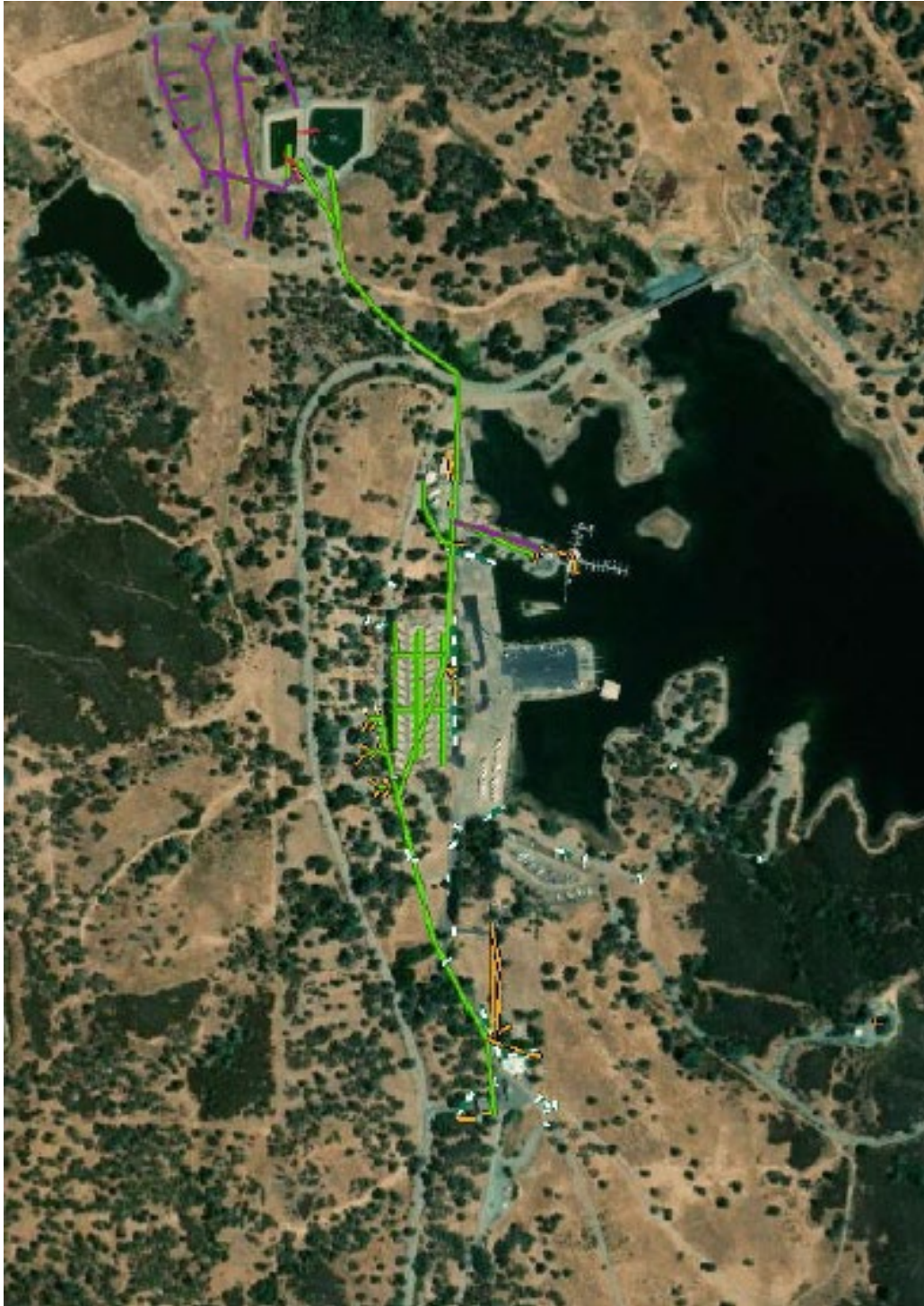
PARA Wastewater System - yellow = sewer laterals, green = sanitary sewer lines, and purple = force main, including effluent application to sprayfields, i.e., purple lines by the wastewater treatment ponds
