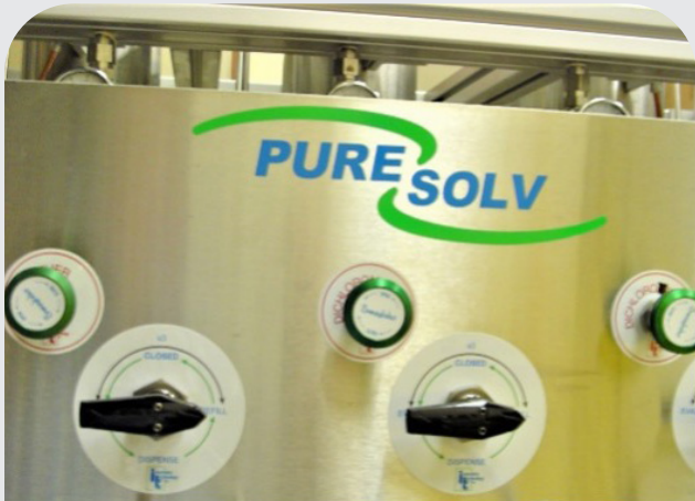
Figure 11-11: Desiccant Drying System for Solvent Recovery
