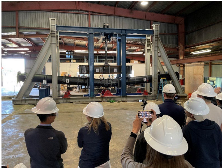
Figure 21. EBMUD employees observe 4-point bending test on a 24" pipe with fiber optic sensors at UC Berkeley Center for Smart Infrastructure.
