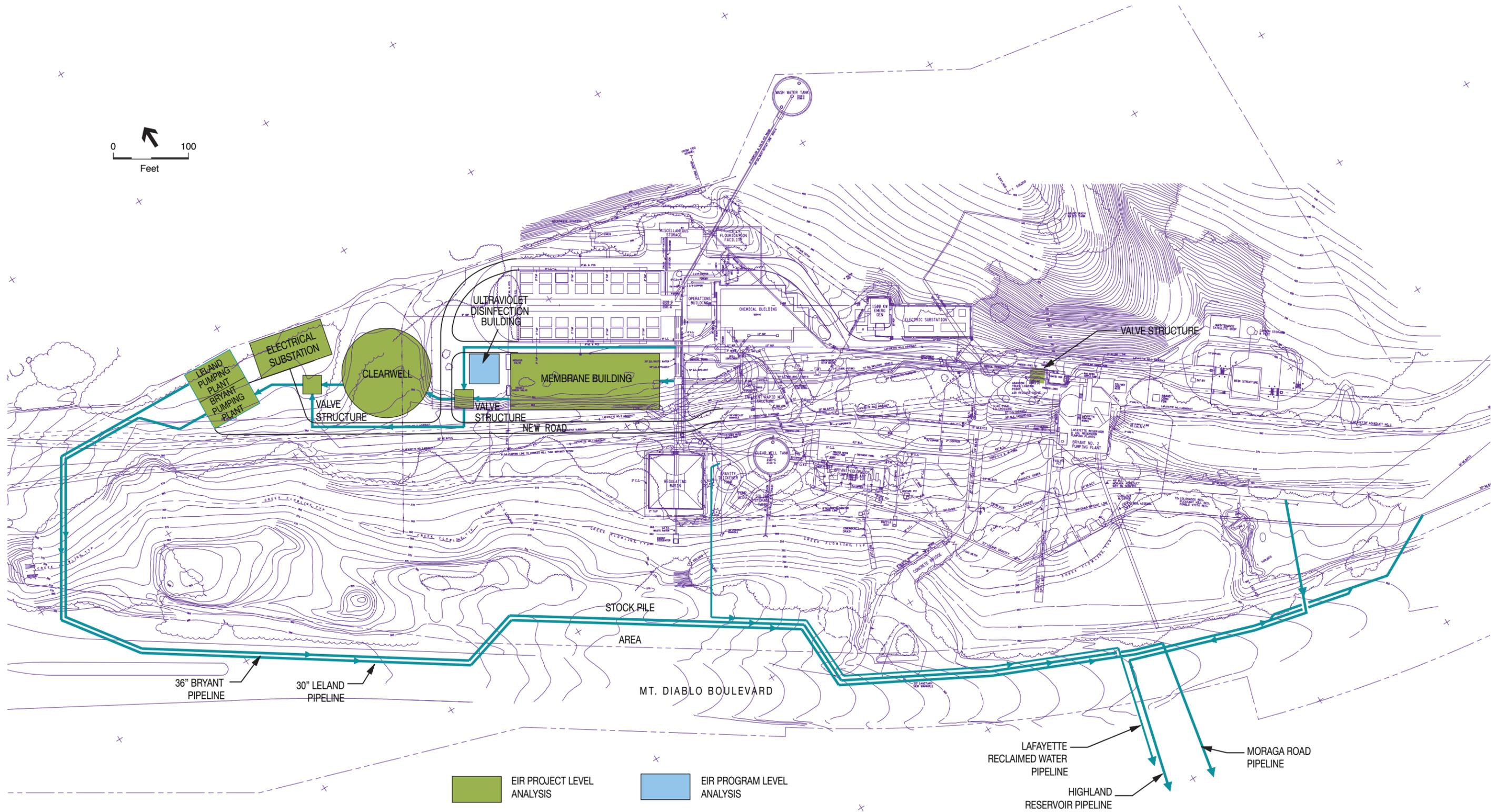
There would be numerous changes to piping within the site, and a new electrical substation would be constructed. The substation would be configured to supply the added power needs associated with membrane filtration processes.
