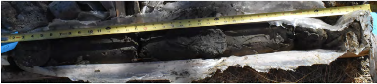
Photograph 10: Boring SB-2 from depth 10 to 15 feet below ground surface
