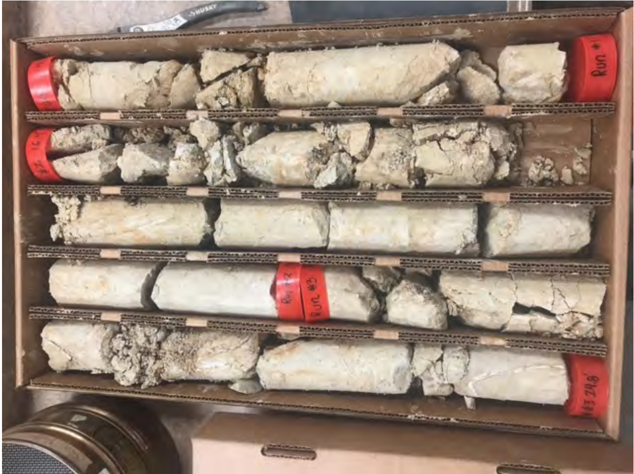
Photograph 18: Boring NMB-1 Run 1 from depth 14.8 to 16.5, Run 2 from depth 16.9 to 21.5, and Run 3 from depth 21.5 to 26.5 feet
