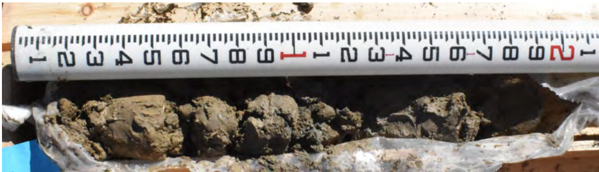
Photograph 12: Boring SB-2 from depth 17 to 20 feet below ground surface
