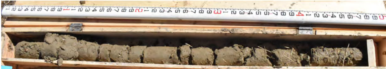
Photograph 13: Boring SB-2 from depth 20 to 25 feet below ground surface
