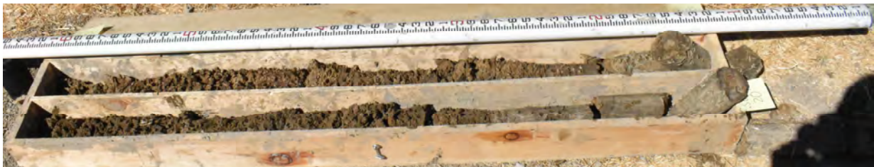
Photograph 4: Boring SB-1 from depth 15 to 20 feet below ground surface
