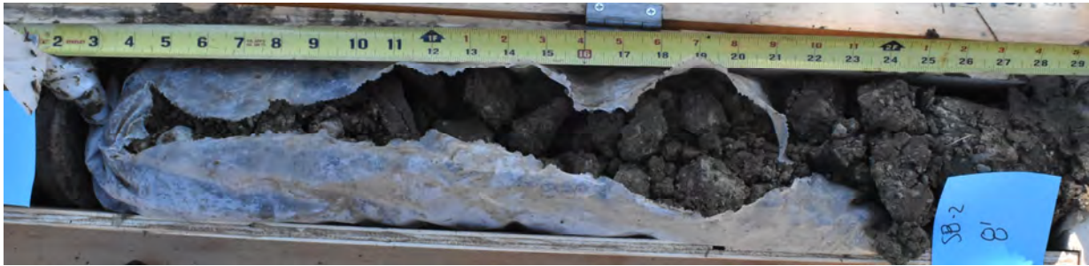
Photograph 8: Boring SB-2 from depth 1.5 to 5 feet below ground surface
