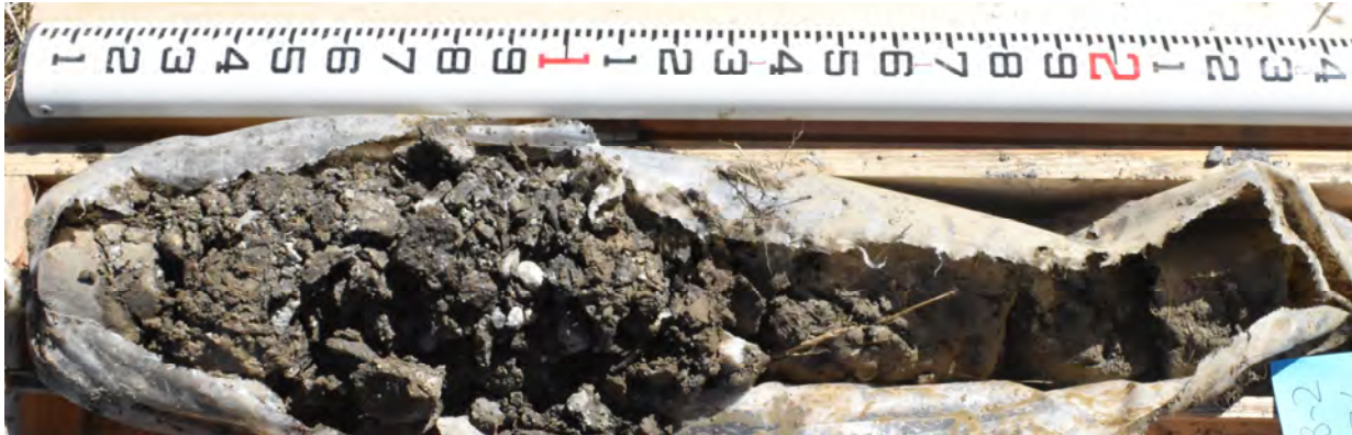
Photograph 11: Boring SB-2 from depth 15 to 17 feet below ground surface
