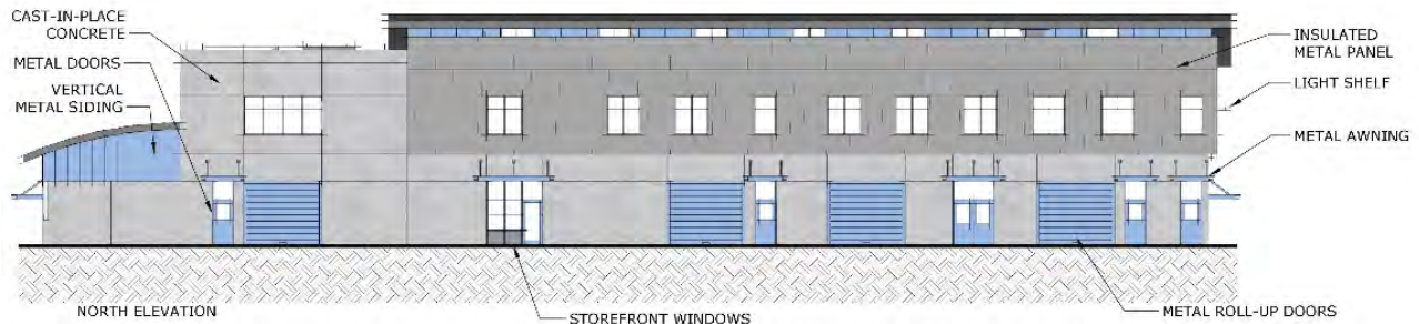
Figure 103- Consolidated Maintenance Building North Elevation
