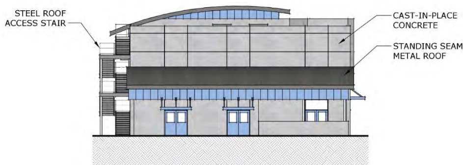
Figure 102- Consolidated Maintenance Building East Elevation
