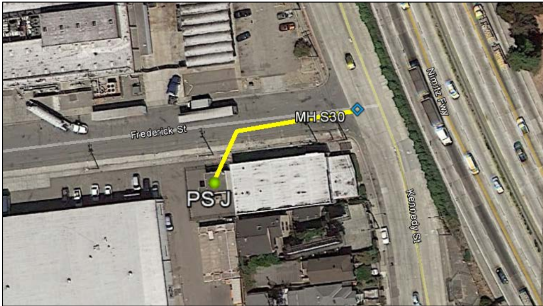
Figure 4-11. Pump Station J and Discharge Pipeline Alignment
