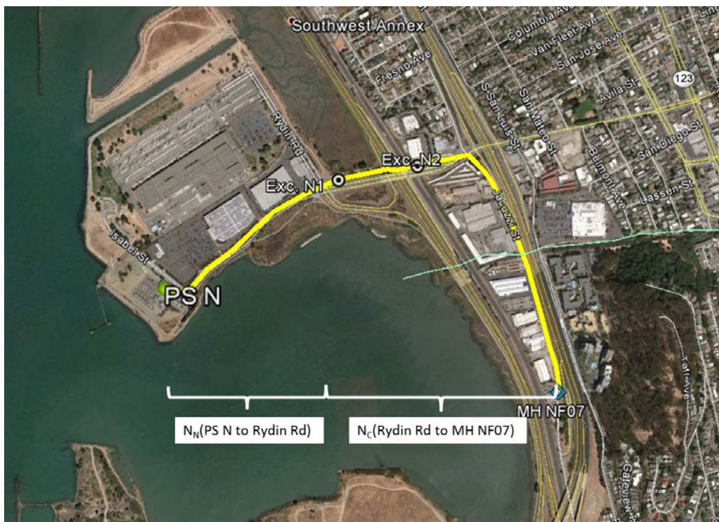
Figure 4-3. Pump Station N and Discharge Pipeline Alignment
