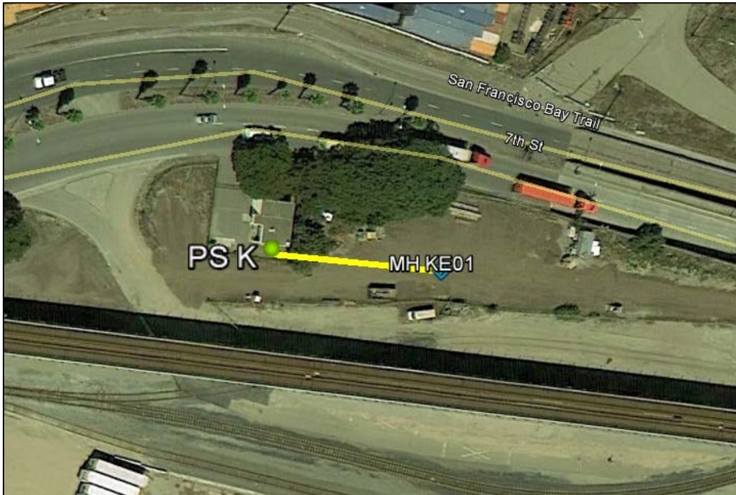
Figure 4-13. Pump Station K and Discharge Pipeline Alignment
