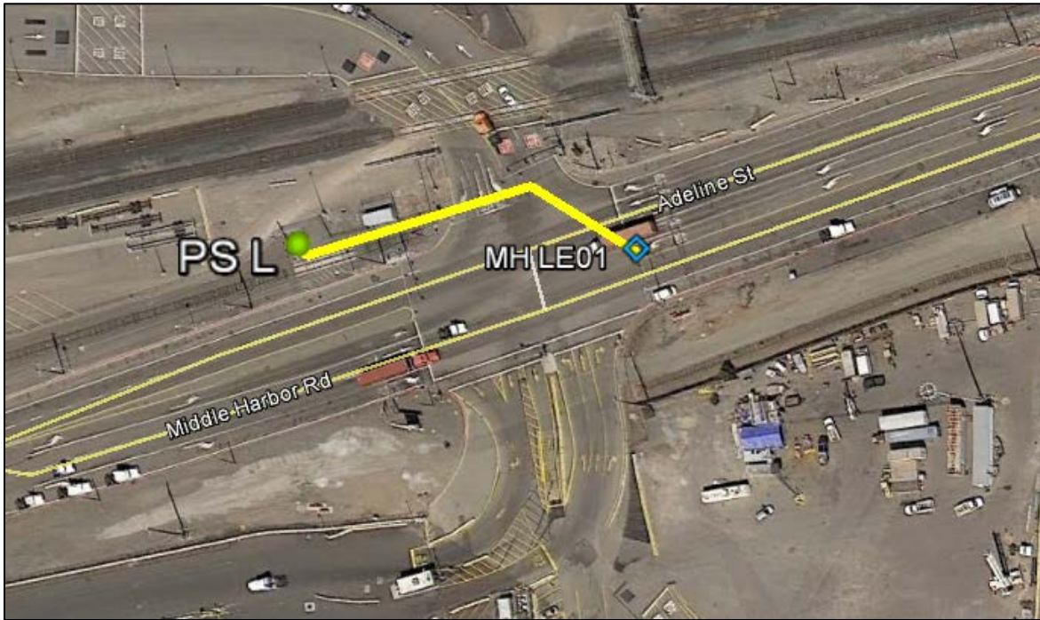
Figure 4-15. Pump Station L and Discharge Pipeline Alignment
