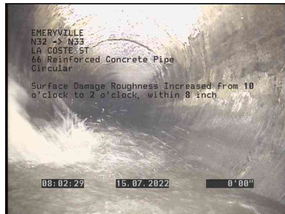
4, 00:01:39, 0.00ft Surface Damage Aggregate Visible from 8 o'clock to 4 o'clock, within 8 inch, Start
