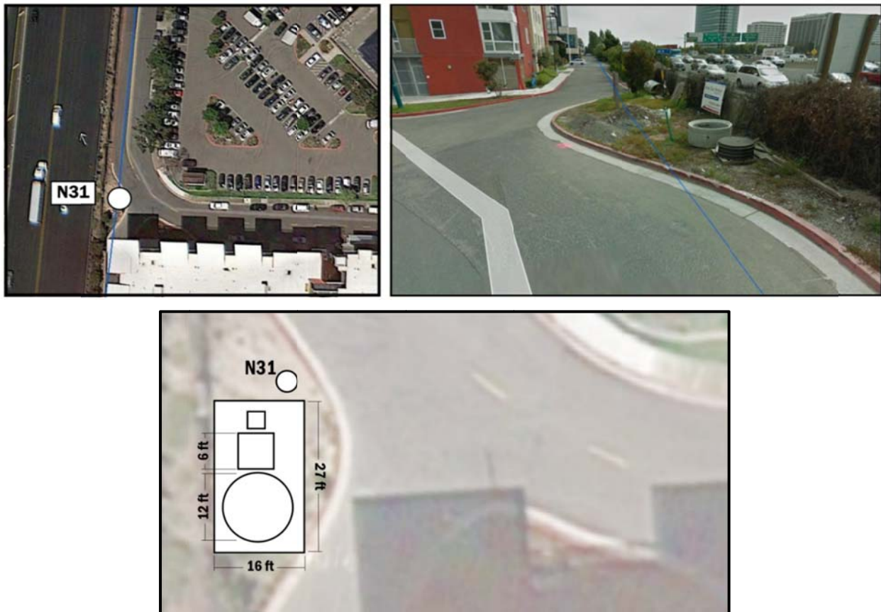
Figure 4-1. Potential Hot Spot 1 Ferrous Chloride Injection Location (Manhole N31)
