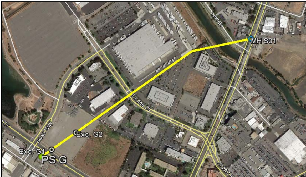
Figure 4-7. Pump Station G and Discharge Pipeline Alignment
