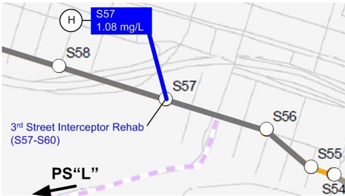
Figure 2-17. Hot Spot 9 (South Interceptor): S54-S57
