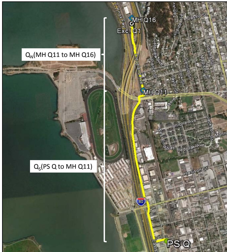
Figure 4-5. Pump Station Q and Discharge Pipeline Alignment
