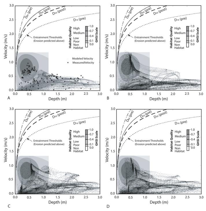
Figure 8 Design phase velocity vs. depth plots at 11.46 cumecs. (A) Pre project. (B) Design scenario 5 (flat riffle). (C) Design scenario 6 (constricted pools). (D) Design scenario 12 (complex channel geometry).
