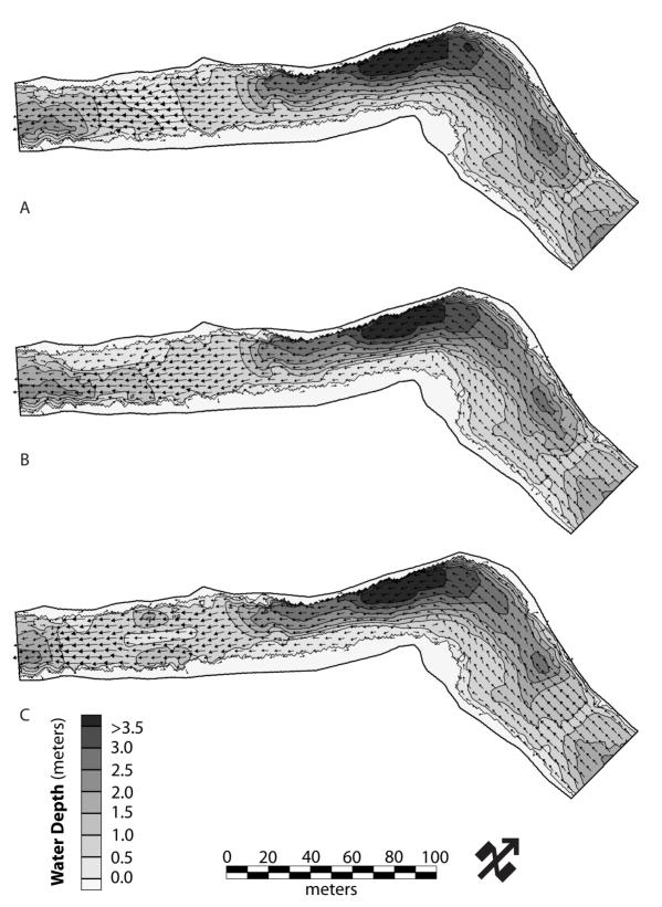
Figure 5 Design Phase Hydrodynamic Model Results at 11.46 cumecs. Shading corresponds to depth solutions and arrows correspond to velocity vectors (scaled to magnitude). (A) Design scenario 5 (flat riffle). (B) Design scenario 6 (constricted pools). (C) Design scenario 12 (final design – complex channel geometry).
