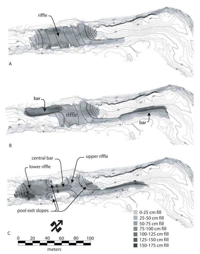
Figure 2 Conceptual designs and grading plans for selected design scenarios. (A) Design scenario 5 (flat riffle). (B) Design scenario 6 (constricted pools). (C) Design scenario 12 (final design – complex channel geometry). Shaded areas represent depth of design specified gravel placement; whereas faded contours represent pre project topography.
