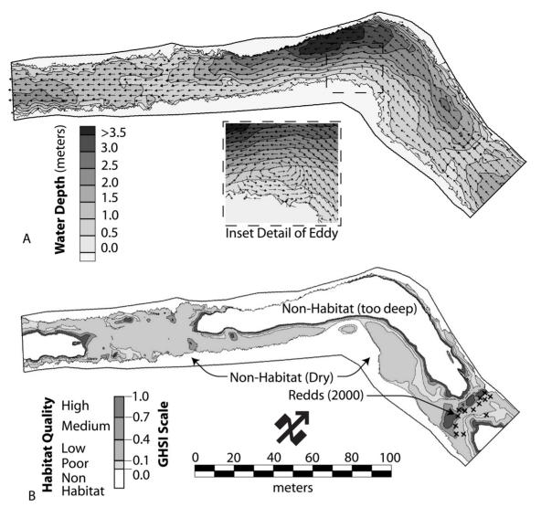
Figure 3 Pre-project Model Results at 11.46 cumecs for comparison. (A) Hydrodynamic Model Results. Shading corresponds to depth solutions and arrows correspond to velocity vectors (scaled to magnitude). (B) Spawning habitat suitability model (GHSI) results w/2000 redd survey results overlaid (redds delineated by black x's).
