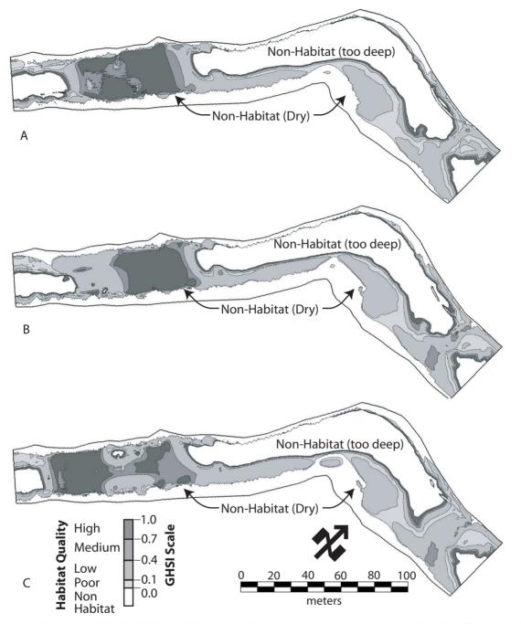
Figure 6 Design Phase Spawning Habitat Suitability Model (GHSI) results at 11.46 cumecs. (A) Design scenario 5 (flat riffle). (B) Design scenario 6 (constricted pools). (C) Design scenario 12 (final design – complex channel geometry).
