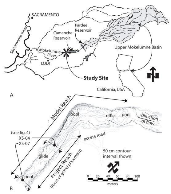
Figure 1 Study site maps. (A) Mokelumne River catchment location map. (B) Topographic survey of study reach showing extent of model domain versus project domain.
