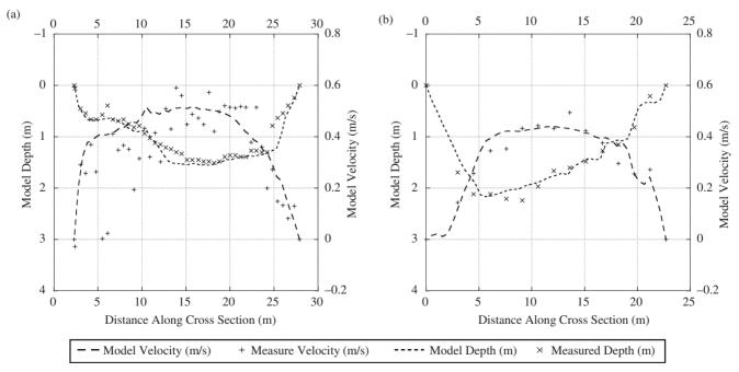
Figure 4 Examples of Pre-project Model validation at two cross sections. (A) Cross section four. (B) Cross section seven. (See Figure 1 for cross section locations.) Generally, poor velocity validation is attributed to areas of poor topographic quality (indicated by errors in measured and predicted depth) and to a lesser extent local-scale measured velocity fluctuations are muted by the model.
