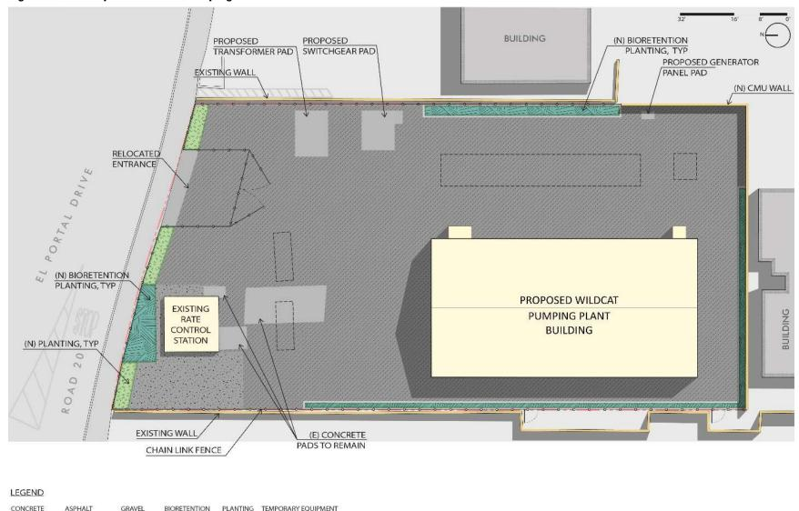
Figure 3 Proposed Wildcat Pumping Plant Site Plan
