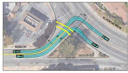
Figure 12 Turning Assessment of a Shifted Centerline at the Road 20/El Portal Drive Intersection
