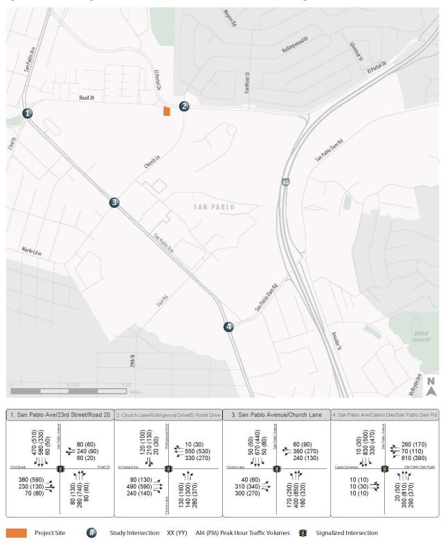
Figure 4 Existing (2021) Peak Hour Intersection Volumes, Lane Configurations and Traffic Controls
