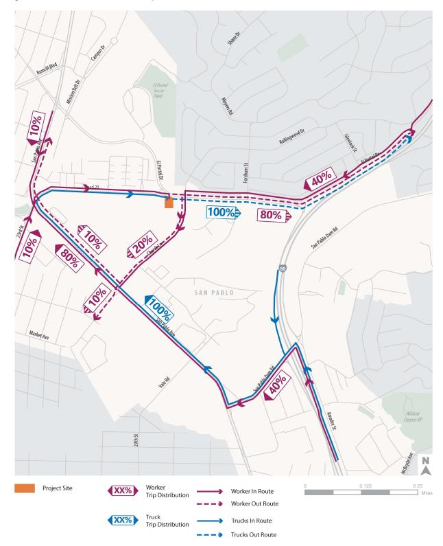
Figure 8 Worker and Truck Trip Distribution
