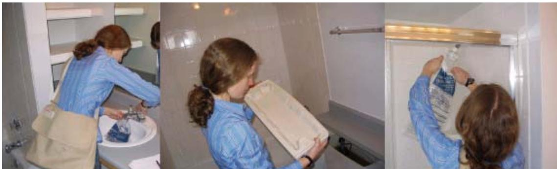
**Figure 3.3 From left to right: a site auditor testing the faucet flow rate, inspecting the toilet lid for a date stamp, and testing the shower flow rate.**
