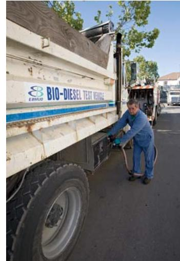
**A new pilot program converts fats, oils and greases from restaurant waste to produce a quality biofuel for EBMUD vehicles.**
