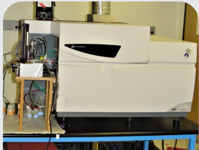
Figure 11-12: Mass Spectrometer Requiring Deionized Water for its Cooling Loop and Connection to Building System Chilled Water Loop
