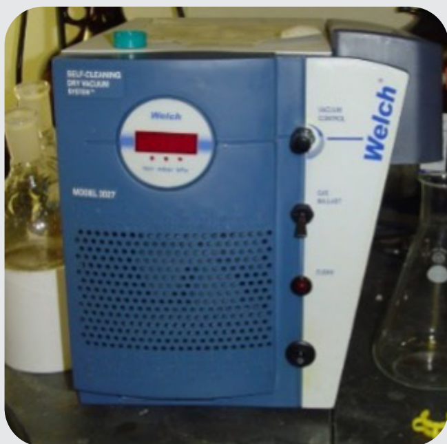
Figure 11-6: Dry Laboratory Vacuum Pump for Chemical and Biological Work
