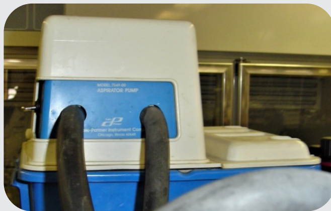
Figure 11-3: Recirculating Venturi Vacuum System
