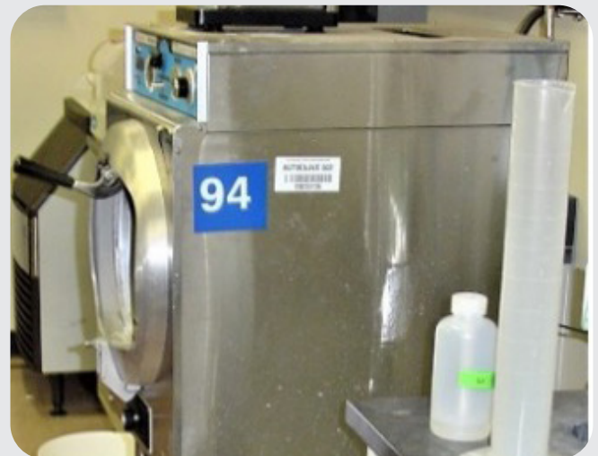
Large Steam Sterilizer at a Laboratory to Sterilize Primate Cages
