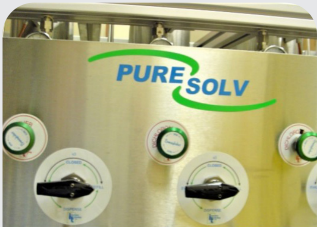
Figure 11-11: Desiccant Drying System for Solvent Recovery
