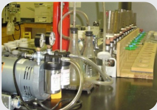
Figure 11-5: Dry Vacuum System in Water Quality Laboratory
