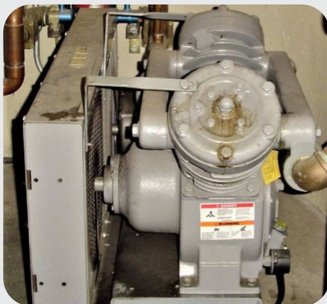
Reciprocating Piston Air-cooled Laboratory Compressor
