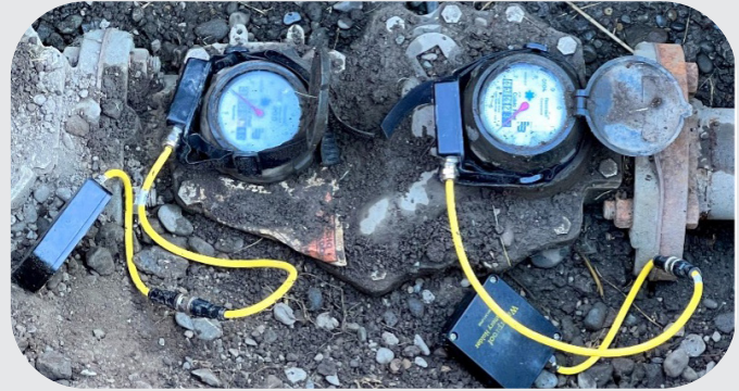
Data loggers on two water meter dials
