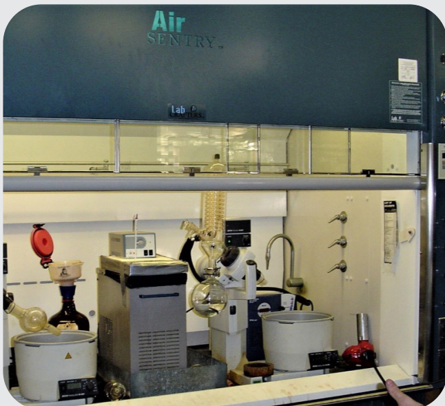
Laboratory Hood with Equipment Using Both a Dry Vacuum Pump and Recirculating Chiller
