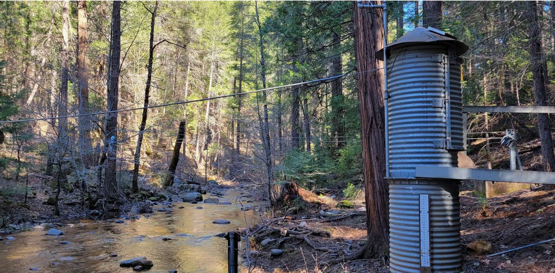
Forest Creek Streamflow Gauging Station, Photo: Jessica Woods
