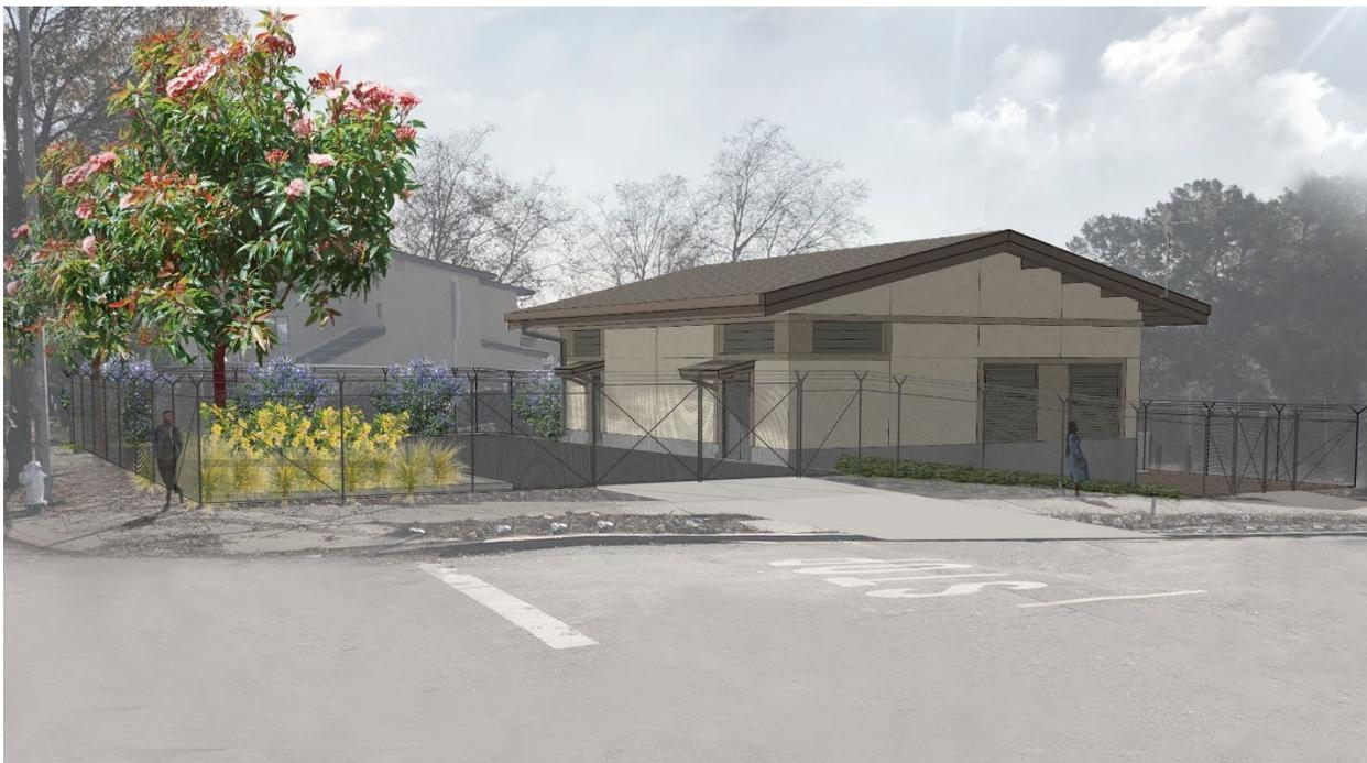
EBMUD selected Concept 2, the Residential Design concept, as the preferred architectural concept for the Fontaine PP building. The concept features beige stucco cladding with contrasting trim over cast-in-place concrete walls, covered by a steel-framed gable roof with brown asphalt shingles. This concept was determined to best meet EBMUD's design objectives and the community's aesthetic preferences.
