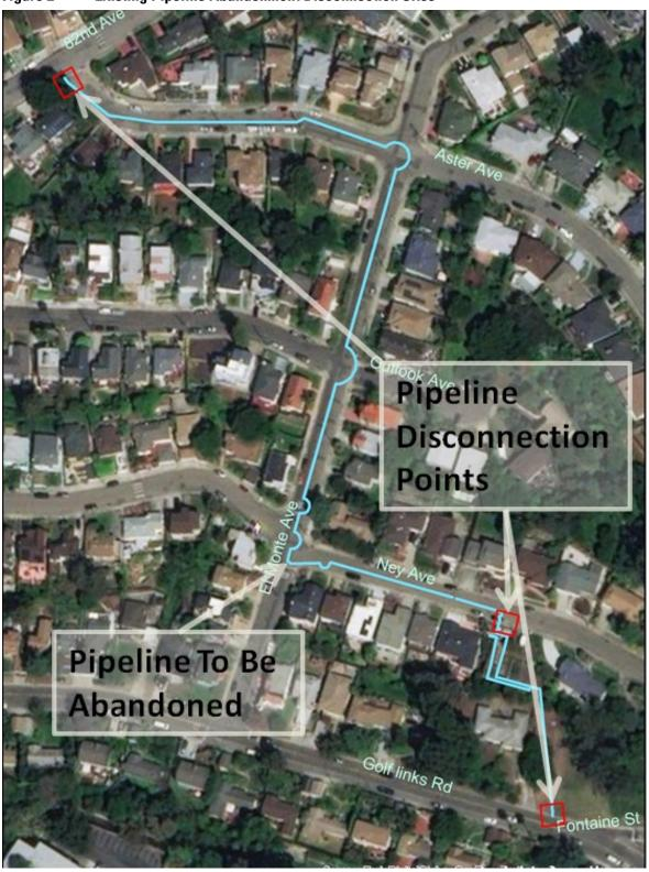
Figure 2 Existing Pipeline Abandonment Disconnection Sites
