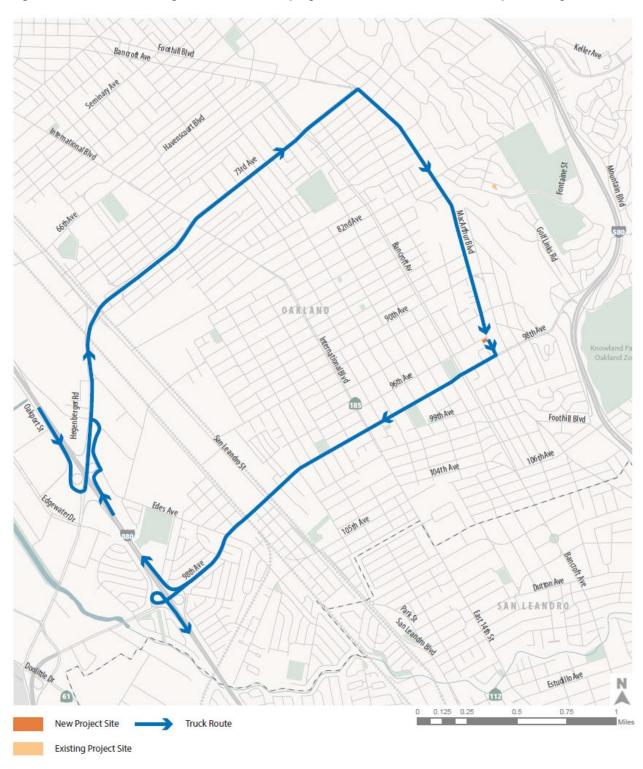
Figure 11 Truck Routing Plan for New Pumping Plant Construction and New Pipeline Alignment
