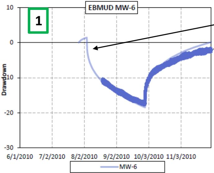
Narrow pale lines are model results and heavier points are the drawdown data recorded during the aquifer test.
