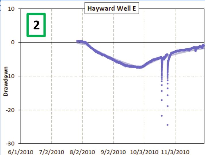
Narrow pale lines are model results and heavier points are the drawdown data recorded during the aquifer test.
