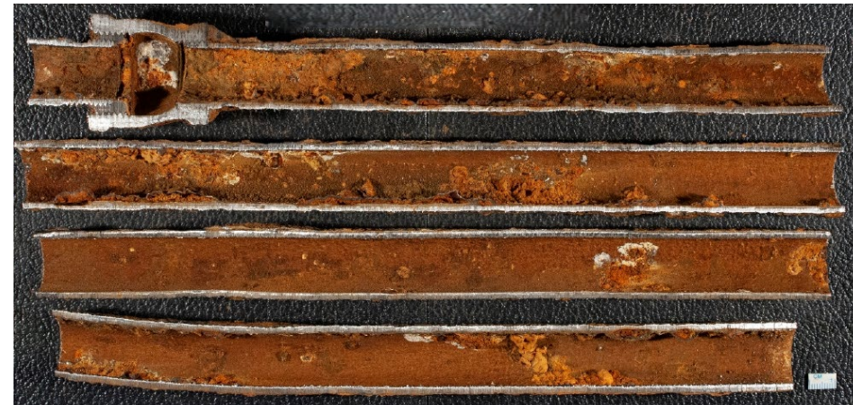
Galvanized pipes after slicing open
