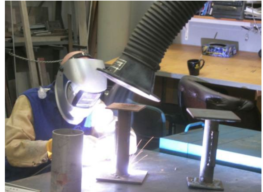
Welding fume monitoring
