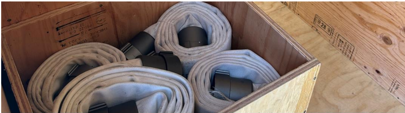
Manifold hose, rolled for proper storage inside trailer
