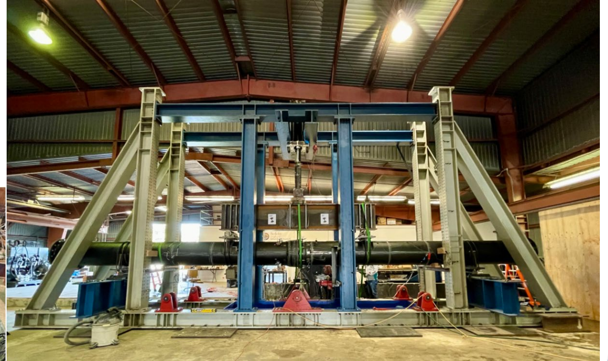
Four-Point Bending Testing Apparatus
