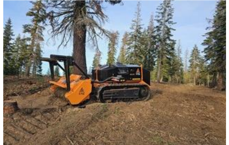
BurnBot remote controlled device performs fuel reduction work.
