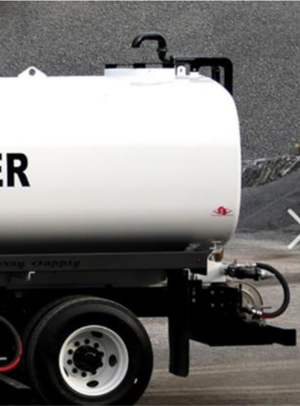
Air gap on water tank
