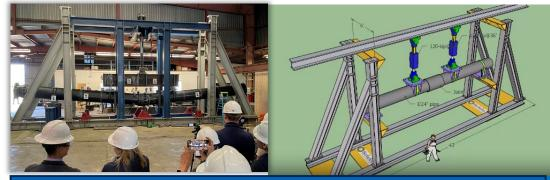
Large Scale Four-Point Bending Testing
