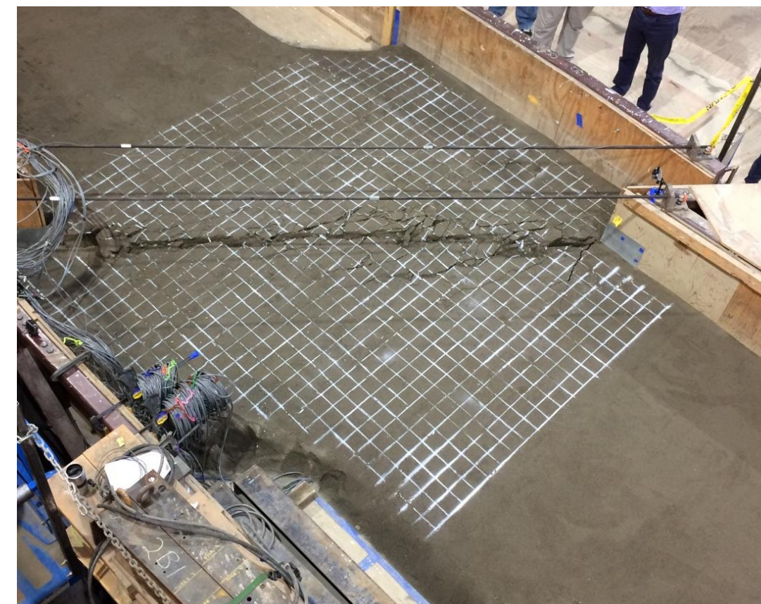
CSI Fault Rupture Test
