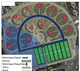
Figure A: East Bay Municipal Utility District Main Wastewater Treatment Plant layout and split-plant configuration. Side A and Side B operate at high and low mean cell residence times, respectively, during split-plant testing.
