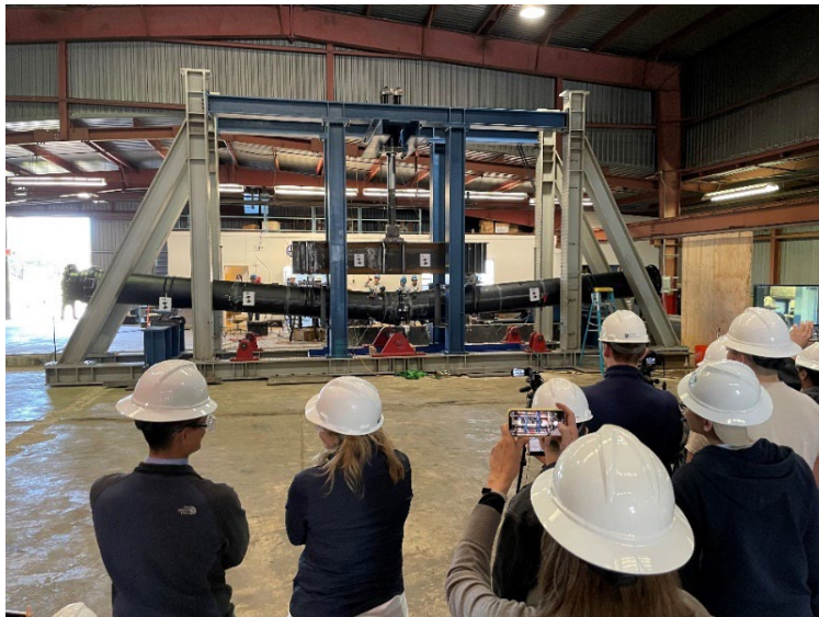
Figure 22. EBMUD employees observe 4-point bending test on a 24" pipe with fiber optic sensors at UC Berkeley Center for Smart Infrastructure.
