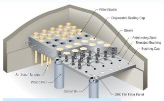
New Robust Filter Underdrain Design
