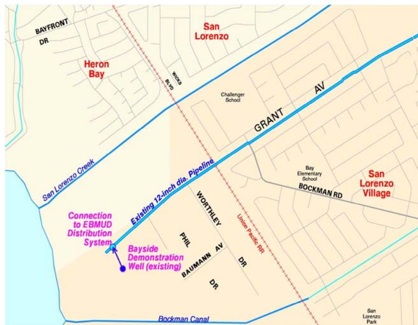
**(Existing) Demonstration Well.** Under Phase I, EBMUD will prepare the existing demonstration well described above for use as a permanent injection/extraction well. Access to the well would be from Grant Avenue through the OLSD treatment plant.
