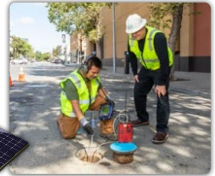
*EBMUD crews deploy acoustic leak detectors to identify and locate leaks in our system.*
